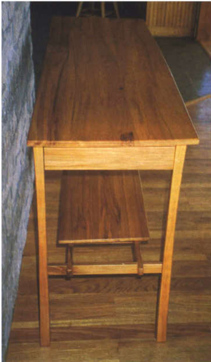
End view of Pier Table shows close fitting drawer front side clearance.
