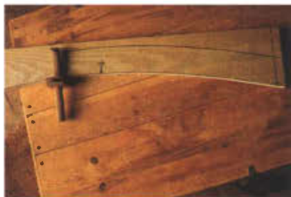
Photo 4. Use a marking gauge to define the 3" width of the arc.
