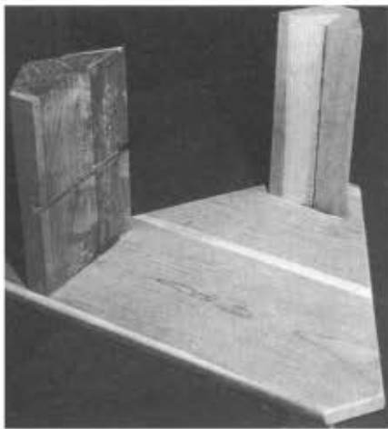
Drawer section above shows left side (G) and back (H) blocks placed. Note dado cut for drawer support (I). Section will later be covered with \frac{1}{4} " solid cherry "veneer."
