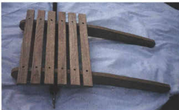
Photo 9. Continue assembling the slats maintaining a ⅜" gap between each slat.
