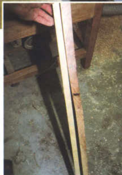
Photo 1. Inspect boards for end checks as shown above. Usually, these ends should be cut off before jointing begins.
