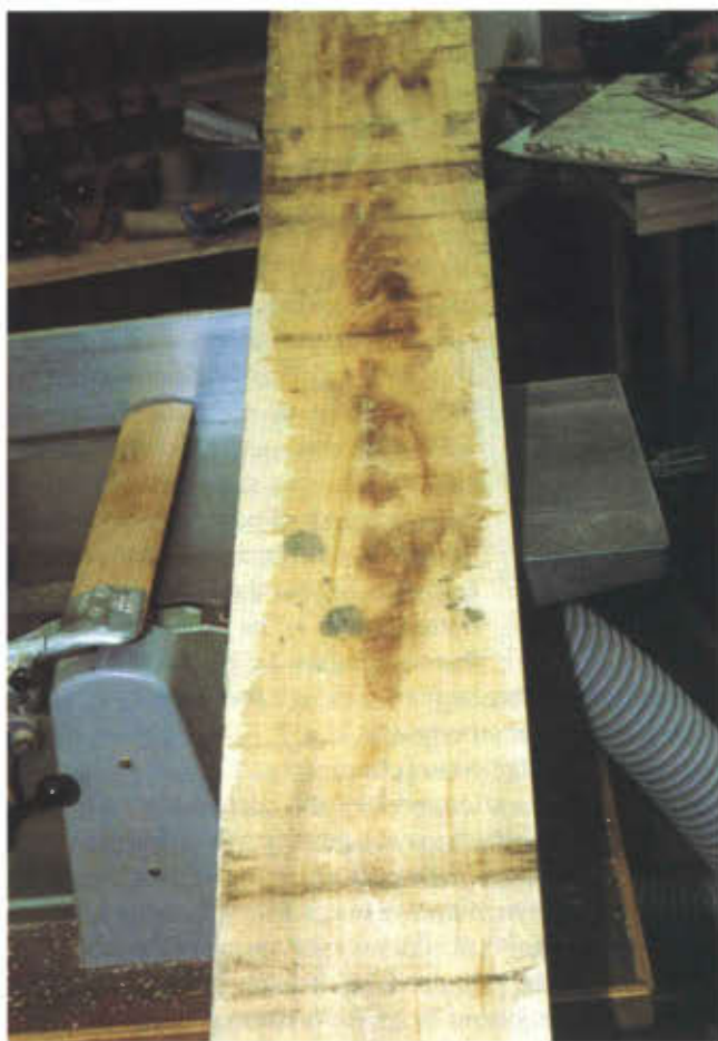
Photo 4. With the cup side down, the first pass on the jointer may only take off material from edges as shown above.
