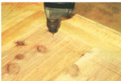
Pre-drilling up through the bottom.
