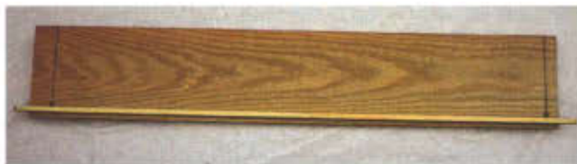
Photo 1. Making the back arc starts with marking a straight line 1" from the edge.
