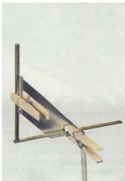
Figure 6. Clothes pins make convenient clamps when soldering
