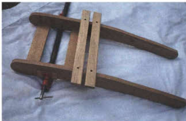
Photo 8. Start attaching the slats 15¼" down from the non- tapered edge.
