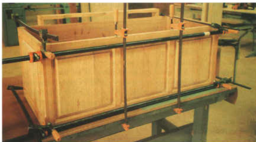
The case assembly in clamps were left overnight to allow the glue to thoroughly set.
