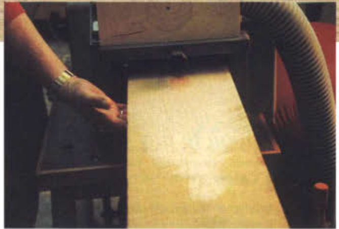
Photo 7. Continued planing takes more material off the higher or thicker areas of the board. Continue planing this face until the board is smooth.
