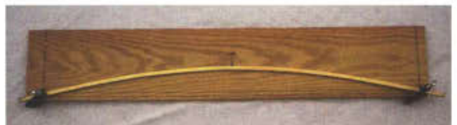
Photo 2. After marking the center and 37" marks, lightly clamp the ends.
