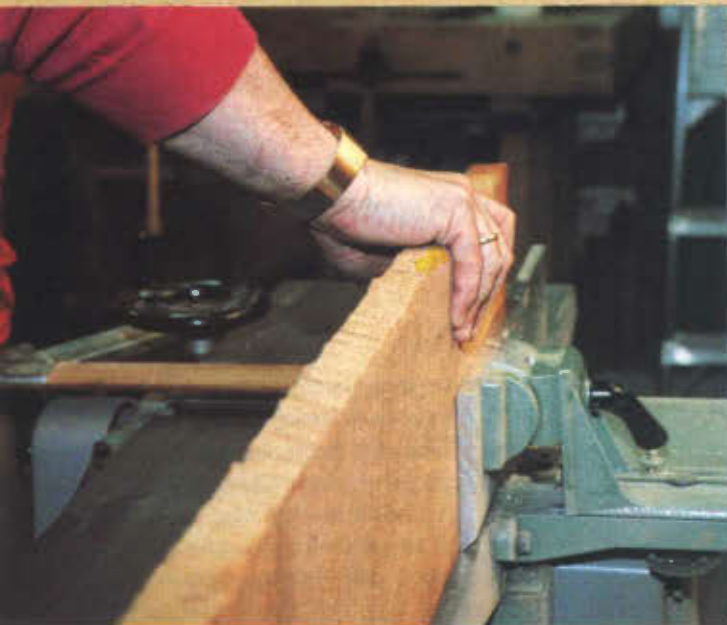
Photo 3. After cross-cutting to rough length, remember to edge joint the stock before face jointing it.
