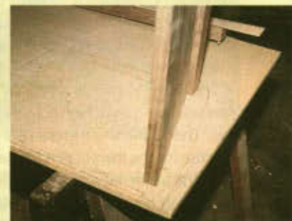
Photo 2. Laying the side on the layout verifies its size and angled end cuts are correct.
