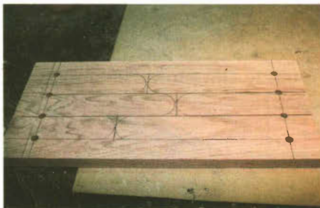
Photo 2. Lay out of the tongues is the most important part of the construction process. This photo shows a six key design.
