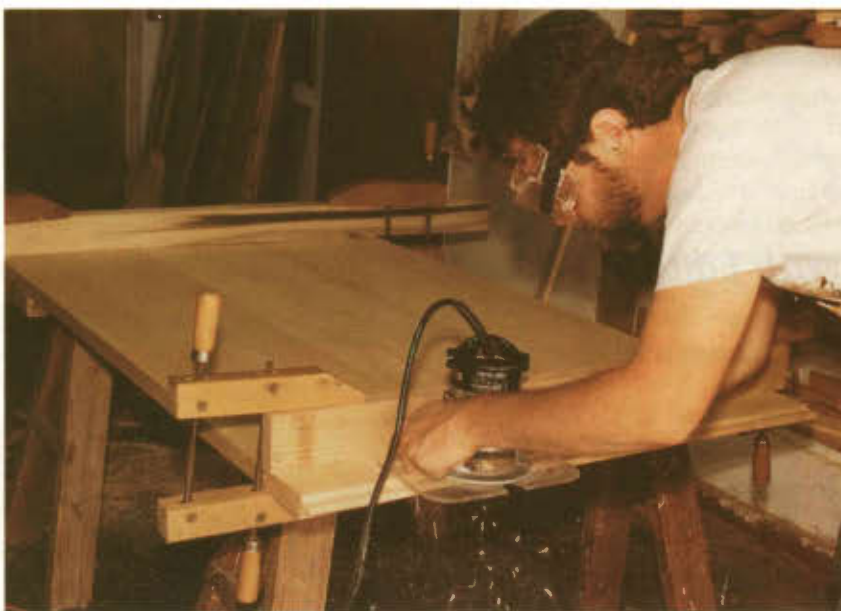
Photo 5. Rout a long tenon on each end of the table top to join the bread board end piece to the top. The tenon was cut from both the top and bottom side of the top.
