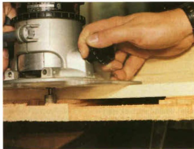
Photo 4. With the table top upside down, fence properly positioned, and shims supporting a board for router base to run on, rout the bottom edges until flush with the thinner middle boards.
