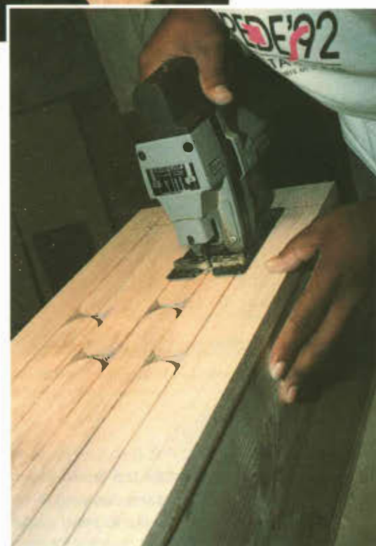
Photo 4. A jig saw is used to widen the narrow bandsaw kerfs.
