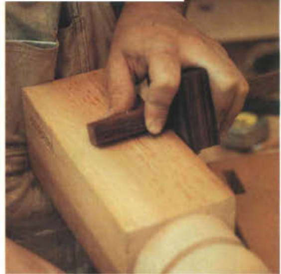
Photo 2. Layout mortise locations on all four sides of leg top making sure opposing faces match.
