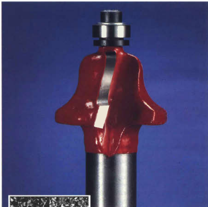
Photo 2. The shear angle of a bit is the angle that the cutting edge makes with the shank of the bit. The bit shown above employs carbide tips angled to slice through wood fibers similar in principal to using a hand plane at an angle to the direction of motion. The slicing action becomes even more important when cutting cross grain. Bits without shear or with too little shear chop the wood and are more likely to produce tear-out and chatter marks. (Information and photo provided by Freud.)
