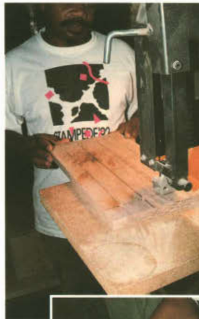
Photo 3. The cuts on the top are done with a bandsaw, cutting first along the length of the tongues, and then dividing the tongues by length. The entry cut at the bridge is later glued back together.
