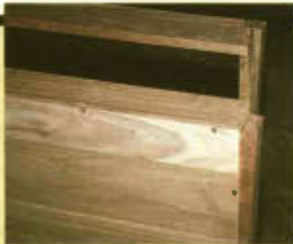
Photo 3. Note rabbets for housing the back and top stretchers. See the relationship between stretchers and legs, front rail.
