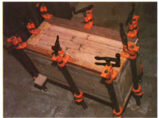
Photo 6. Heavy clamping insures there will be no gaps in the glue joints.
