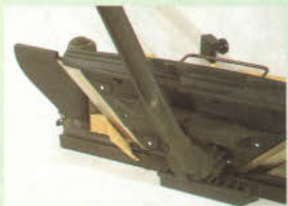
Photo 6 The final cut should always result in see-through shavings that curl away. This will leave an edge that requires no further attention before assembly.
