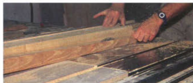
Photo 3 After drilling, the legs were tapered on the table saw.
