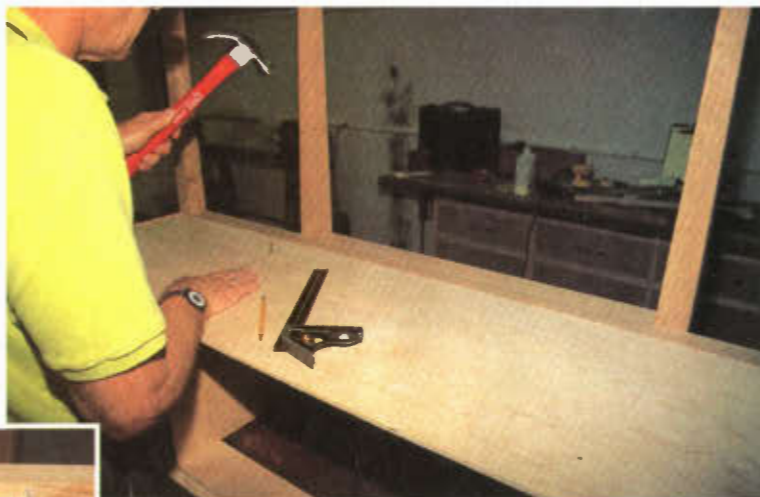
Photo 7 (above) Partitions between drawer and door sections are nailed up through the bottom and down through the front and back stretchers.
