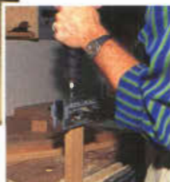
Photo 2 (right) The front rail ends were drilled using a doweling jig.
