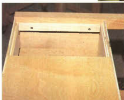
Photo 6 (above) The cabinet sides are glued to the legs using biscuits to align. The side setback from the leg is created by simply adding a 1/4" spacer under the biscuit joiner fence when cutting the side slots.
