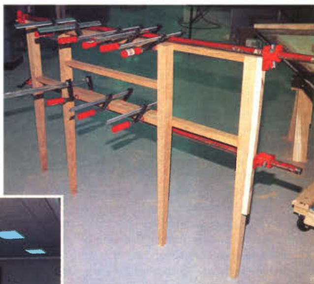
Photo 4 (left) The step out drawer section, leg and rail assembly is glued with dowel joints and clamped. The diagonal clamp is used to pull the assembly square while the glue dries.
