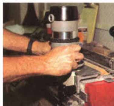
Photo 9 Half blind dovetails routed on a jig were used for drawer construction. Another method would be to rabbet the front and back to receive the sides.
