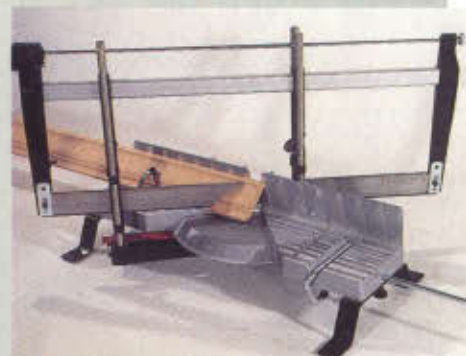
Photo 2 Compound miter cuts are accomplished by tilting the work against the fence. Grooves in the bed provide the position for slope angles of 20°, 30°, 40°, 45°, 50°, 55°, and 60°.
