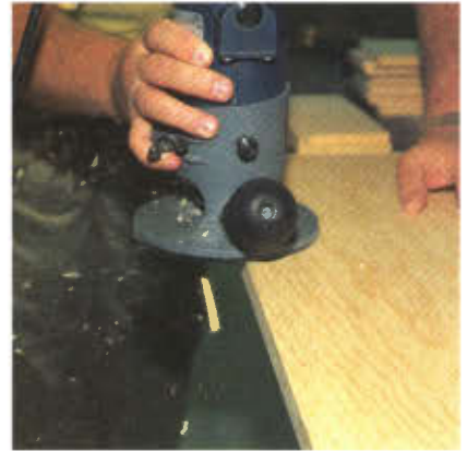
Photo 3 A router with a \frac{1}{4} " x \frac{1}{2} " straight bit makes quick work of cutting the rabbets on the ends and back edge of the top.
