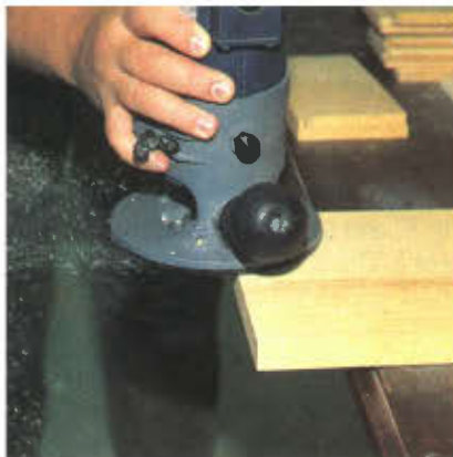
Photo 6 Easing or breaking most of the exposed edges with an \frac{1}{8} " roundover bit quickly removes sharp edges and adds a simple detail.
