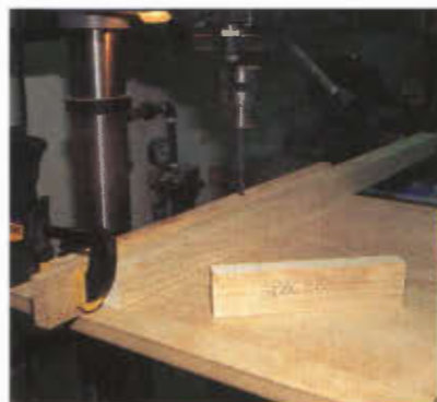
Photo 2 (right) The front rail ends were drilled using a doweling jig.
