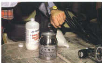
28. The HVLP sprayer comes with a viscosity tester. Follow instructions carefully to make sure the unit sprays the material properly: The Behlen's was just about perfectly mixed right out of the jar.
