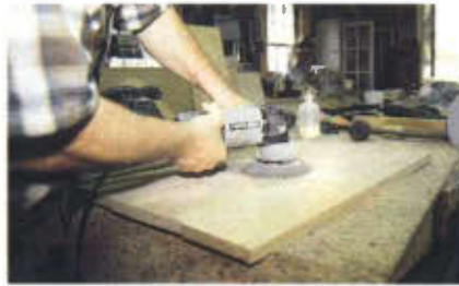
20. Sanding drawer fronts flat. The random orbit sander does an incredible job for a relatively lightweight sander that also will do a superb job of finish sanding.
