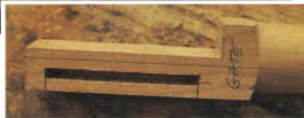
11 & 12. Before and after views (above and right) of cutting away the excess material from the gate leg so it will close accurately against the apron rail.
