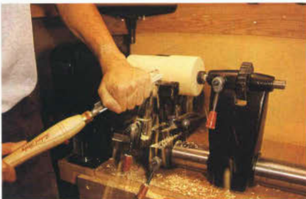
Roughing blank between centers.
