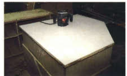
26. Trimmed laminate on the corner section.
