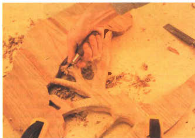
(Photo 8) Undercutting the branches from the underside of the blank using the carving knife.
