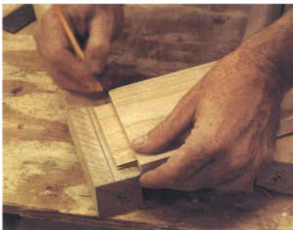
8. Hold-down jig for angle-mortising on the legs.
