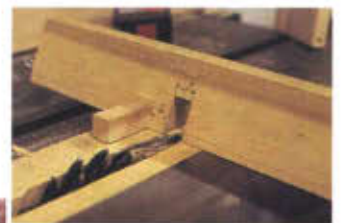
4. Drilling pin-hole for gate (left). 5. Below, detail of the angled screw pockets being drilled in apron for top attachment. 6. Inset shows jig used in making finger joints for gate joint in apron.
