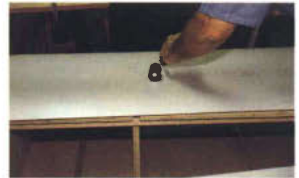
24. A good veneer roller works to force contact.
