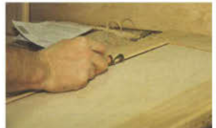
15. The Veritas tool rounds over the inside edges of the door stiles and rails.
