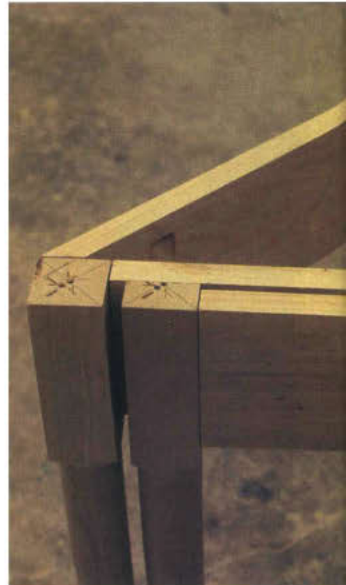
Photo at right shows finished assembly of gate leg and apron in closed position. The next step is staining and finishing.
