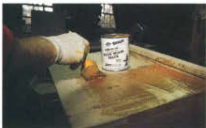
27. Behlen's Pore-O-Pac and water-based polyurethane serve as the total finish. No stain was needed. Use with rubber gloves.
