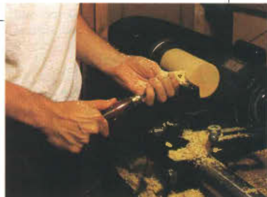
Making preliminary parting cuts as reference lines.
