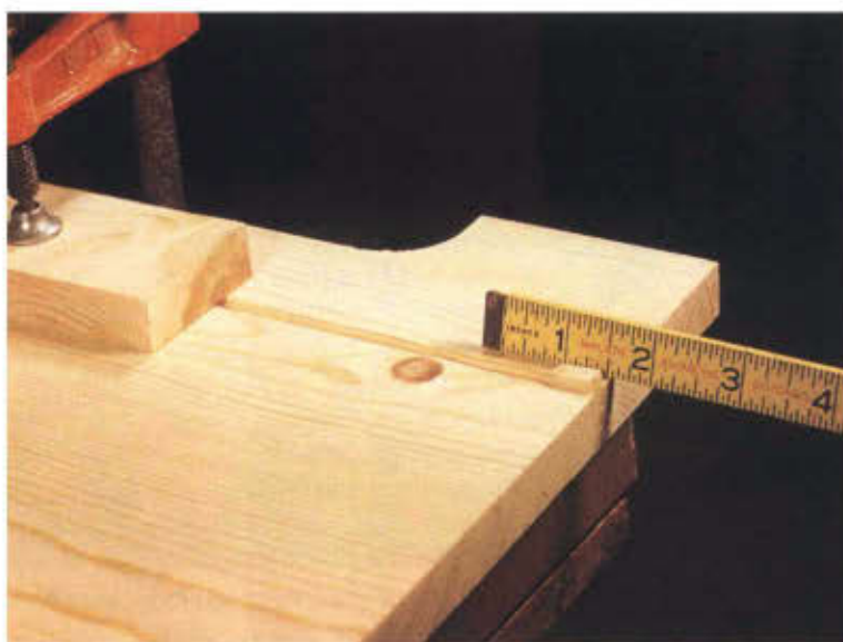
After the 2" holes are drilled on the panels, cut and glue the \frac{3}{8} " wide x \frac{1}{2} " long plug into all slot ends on the front and rear panels to fill the saw cuts.
