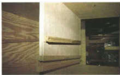
8. Leave the back of the drawer section open when setting drawer guides.
