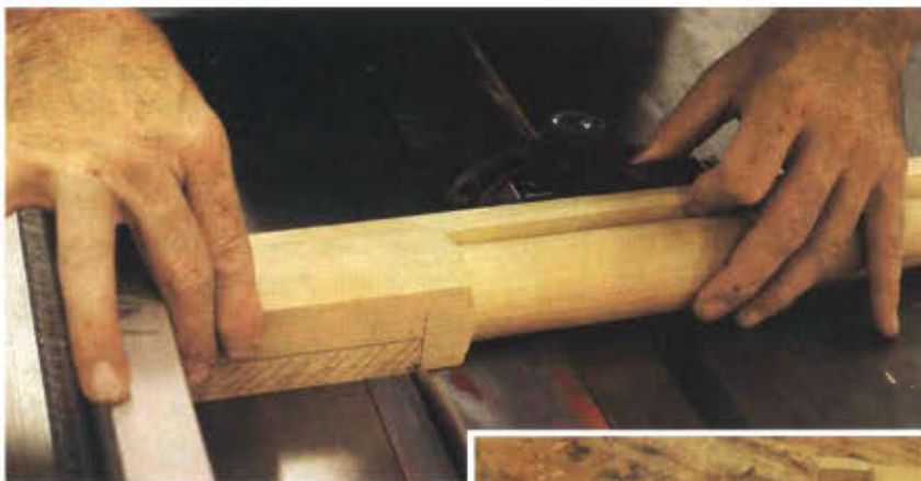
11 & 12. Before and after views (above and right) of cutting away the excess material from the gate leg so it will close accurately against the apron rail.
