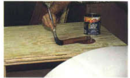
21. Brushing works for contact cement.
