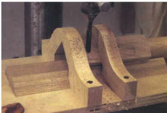
8. Hold-down jig for angle-mortising on the legs.
