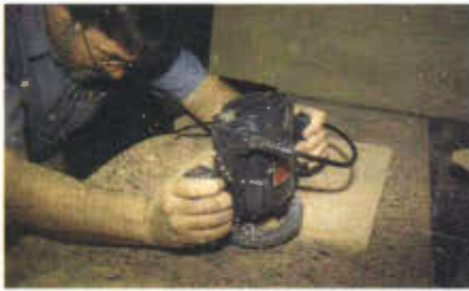
19. Routing the drawer edges.
