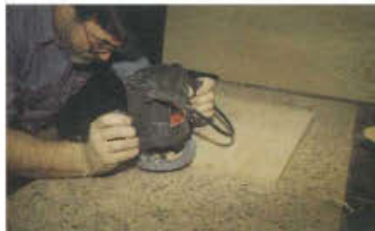
14. Edging the drawers using a roundover bit.
