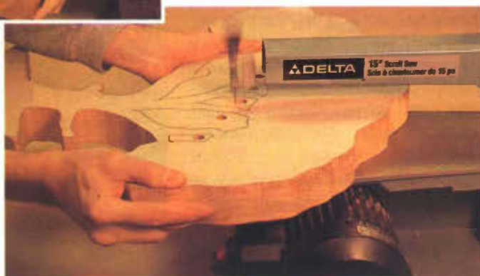
3 Using the scroll saw to cut the waste out from between the branches.
