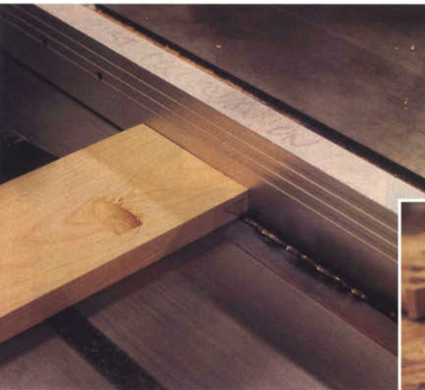
2 & 3. Table set-up and finished view of angled tenon on apron pieces.
