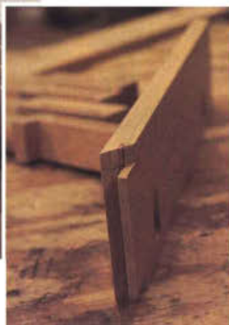
2 & 3. Table set-up and finished view of angled tenon on apron pieces.
