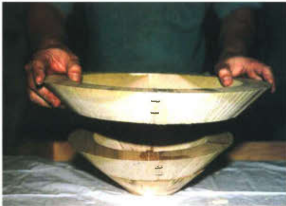
(Photo 4) Make sure each circle is centered on the one below during gluing.
