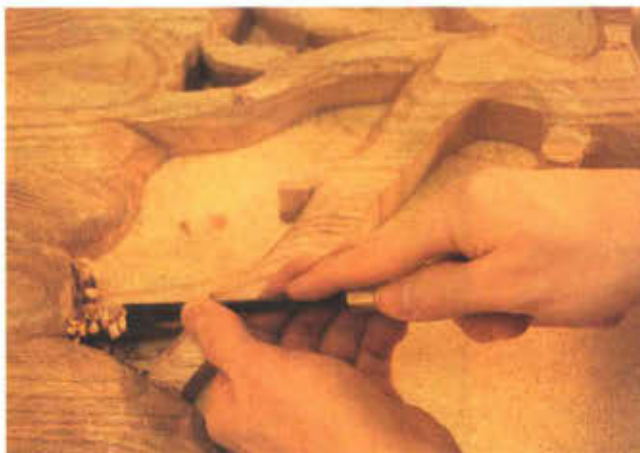
(Photo 6) Paring a branch with 1/2" #6 gouge.
