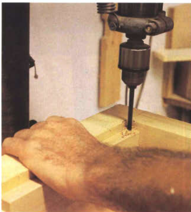
4. Drilling pin-hole for gate (left). 5. Below, detail of the angled screw pockets being drilled in apron for top attachment. 6. Inset shows jig used in making finger joints for gate joint in apron.
