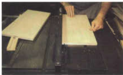
4. Cutting dados for drawer bottoms.
