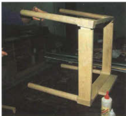
Photo 13. The table base was dry fit prior to gluing the parts.
