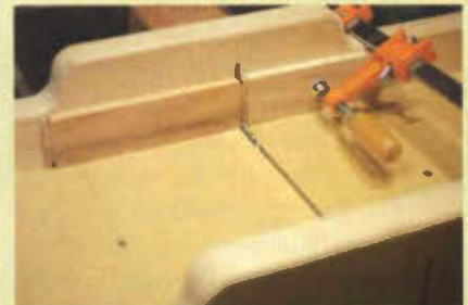
Photo 12 The length of the tenon was milled by cross cutting on the table saw. A gauge block clamped in place assured accurate, repetitive cuts.
