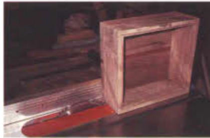
Photo 5. Carefully separate the top of the box from the side using your table saw. Particular care should be taken on the final cut.
