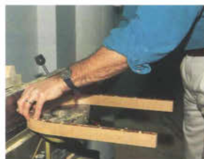
Photos 7 and 8. With the jointer fence moved to the left for safety, the top edge of the part on the form (the edge you could clean the glue from) is jointed flat and square to the side. When jointing, use special caution keeping your fingers on top of the work only. First run the part with the machine turned off to get a feel for the turns and placement of your hands.
