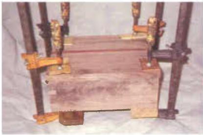
Photo 4. The top is glued and clamped to the assembled box. Notice the scrap boards used to protect the bottom edge of the box.
