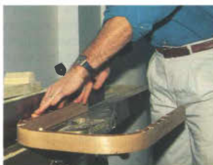
Photos 7 and 8. With the jointer fence moved to the left for safety, the top edge of the part on the form (the edge you could clean the glue from) is jointed flat and square to the side. When jointing, use special caution keeping your fingers on top of the work only. First run the part with the machine turned off to get a feel for the turns and placement of your hands.
