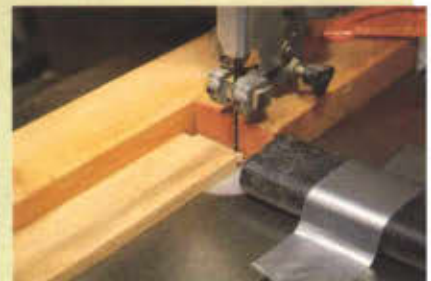
Photo 12 (below) Tenon shoulder waste is trimmed on the bandsaw. A stop block is clamped behind the blade to prevent cutting too deep. A vacuum hose is taped to the saw table to collect dust.
