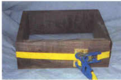
Photo 2. The band clamp shown was used to clamp a corner-mitered version of the humididor. The corner miter offers a simpler version.
