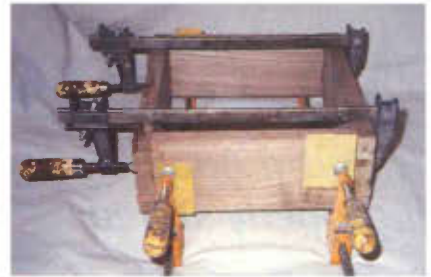
Photo 3. When clamping up the dovetail joints, standard bar clamps are still your best bet for a tight joint.
