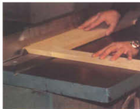
Photo 5. After the face frame has dried, the 45° angle is cut on the stile edges.
