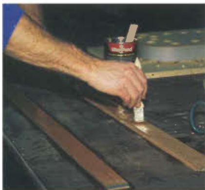
Photo 1. When applying glue to the eight strips to be bent, keep them in a stack after brushing on a moderate amount of glue. By stacking, you slow the drying of the glue, providing more time for clamping on the form.
