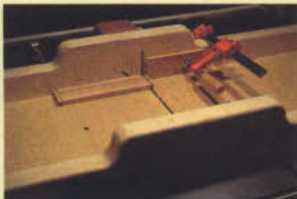
Photo 10 Initially, Andy established the shoulder and prevented tearout by cross cutting on the table saw. When he discovered this step was unnecessary, he went directly to the router table, saving time.
