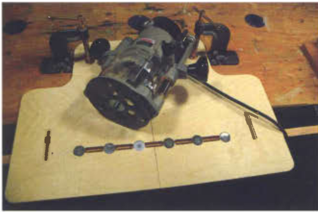
Photo 4 The jig has the fender washers properly placed along the slot. Their accurate spacing, along with the router template guide, will produce the proper sized mortise.
