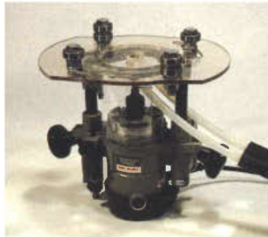
Photo 8 (above) The completed shoe for the vice-mounted jig with two fixed bearings, two adjustable bearings, and other holes for router bit, mounted holes and vacuum holes.
