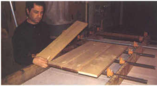
Photo 2. Gluing-up the back panels using solid stock. This allows the option of adding an edge detail between the glued boards.
