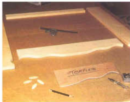
Photo 4. The front face frame is ready for assembly. Note the 45° degree angle on the edges are not cut until after clamping.
