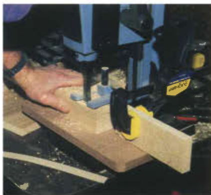
Photo 10. The mortises for the legs were cut using a bench top mortising machine with a \frac{1}{2} " hollow chisel.
