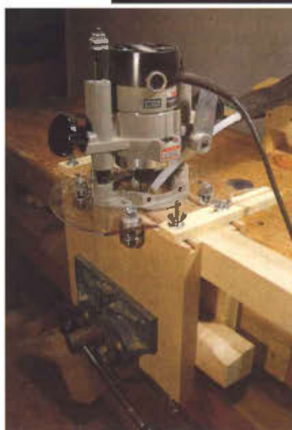
Photo 1 Andy has his slat mortising jig set up and ready to run. Using this and the vice-mounted jig at left, he milled 80 mortises in just 32 minutes.
