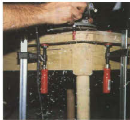
Photo 15. Next, clamp the template in place and trim with a top-mounted bearing flush bit chucked in the router. Avoid tear-out by climb cutting the end grain.
