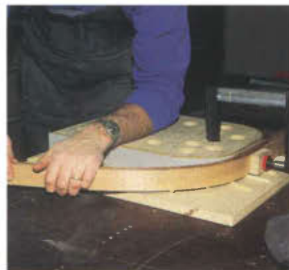
Photo 3. With the top clamp set, pull one side around to the end and loosely set a second clamp. Keep this clamp loose so that the stack can slide through it as other clamps are placed, taking out the gaps.
