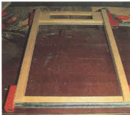
Photo 11 After the dowels are ready, the front and back frames can be assembled.
