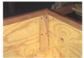
Photo 11 Secure the legs from the inside of the cart after passing through to notched bottom.
