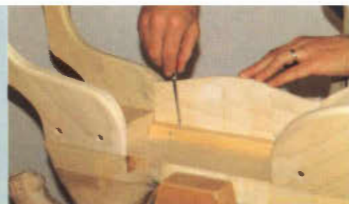
Photo 7 The battens for the body sides are glued and screwed in place.
