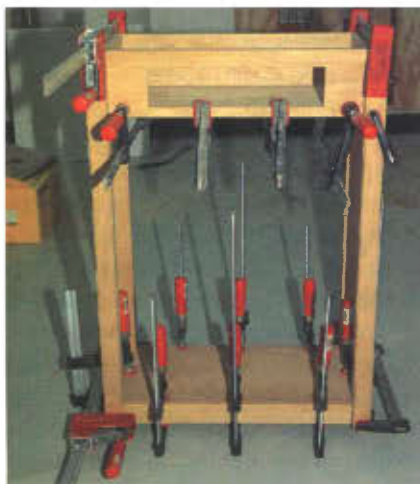
Photo 14 If you have the clamps to do it, the bottom and inside bottom can be glued in place while the frame is drying.
