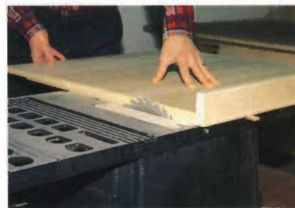
Photo 2 With the table saw panel squaring jig, I squared one corner of each cabinet part then marked it with a pencil.
