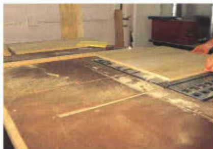
Photo 15 By clamping an auxiliary fence parallel to the blade, the width of cut capacity is greatly enhanced.
