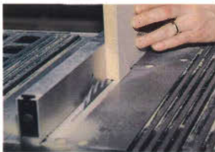
Photo 4 Rabbits are cut running the panel on edge against the fence which is set to \frac{1}{4} " with the blade set about \frac{1}{16} " high.
