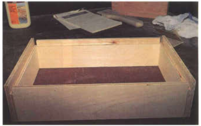
Photo 17 The drawer box uses simple butt joints and a rabbet for the bottom.
