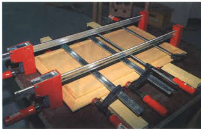
Photo 19 The top's edges are glued in one step to make sure the corner miters are accurate.
