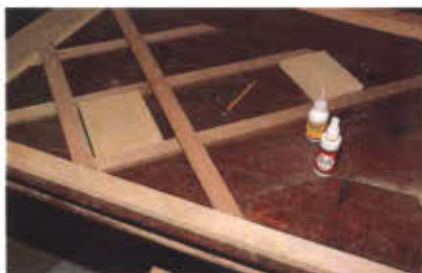
Photo 1 The slat section is glued together using a temporary frame and blocks to determine spacing.
