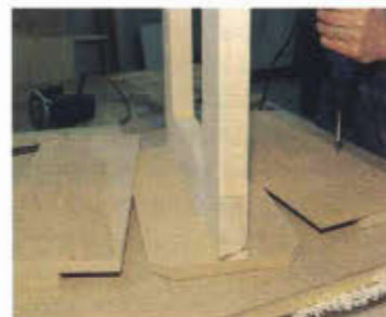
Photo 13 The removable legs of the folding top sleeve into mating parts screwed to the top's underside.
