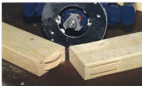
Photo 12 With no biscuit joiner in the budget, a router does the trick. Here double biscuit leg joints are made using a \frac{1}{2} " slot cutter with a \frac{1}{8} " bearing.
