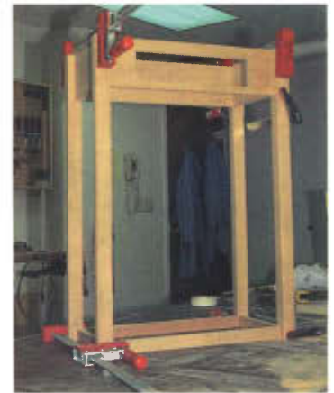
Photo 13 The second frame is then attached and the entire assembly is clamped until dry.
