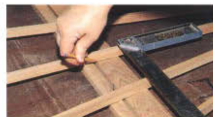
Photo 7 By using the spacer jig, the cross brace spacers are easily marked.
