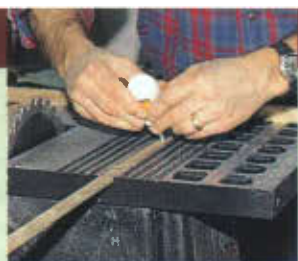
Photo B To space the guides accurately, place them in the slots, apply glue, then set the sled in place.
