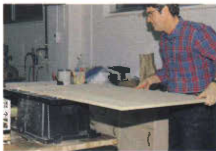
Photo 3 Each panel is trimmed to final size using the saw fence cutting opposite edges to the squared corner.
