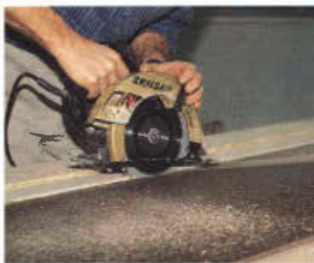
Photo 10 The straight edge saw jig and a plunge cut were used for making cutouts in the top.
