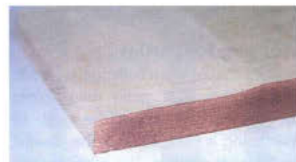
An extreme example of snipe, which can be prevented with proper machine setup, stock preparation and support during planing.
