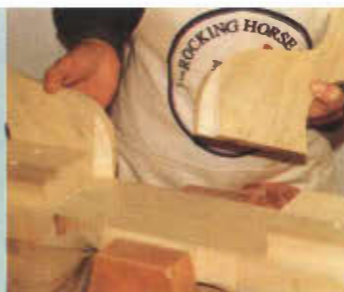
Photo 6 The leg fixing blocks are attached, then the legs are notched to match.
