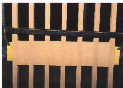
Photo 6 The spacer blocks are glued into place forming the cross brace.
