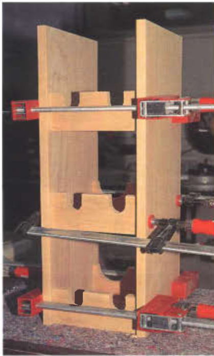
Photo 16 The bottle section is assembled after the height of the partitions has been checked for fit in the server frame.
