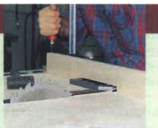
Photo C I clamped boards in place to help align the sled perfectly.
