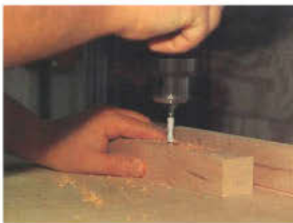
Photo 10 A piece of tape on the drill bit is used to indicate the appropriate depth. Of course, you could set the depth adjustment on the drill press, but that takes all the fun out of it!
