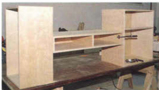
Photo 9 In turn, the general storage cabinet is screwed to the other two while held in place with a clamp.
