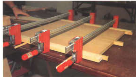
Photo 4 By clamping solid cherry edging to the particle board, the look of solid cherry furniture can be achieved at bargain rates.
