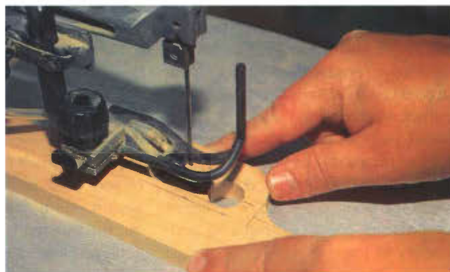
Photo 20 A scroll saw is the perfect tool for connecting the two \frac{3}{4} " holes which form the tray handles.
