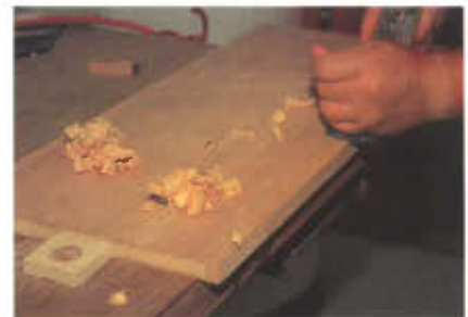
Photo 5 When planing the solid edges flush to the veneered particle board, be careful to keep the plane iron level to the surface. It only takes a simple slip to gouge the veneer.
