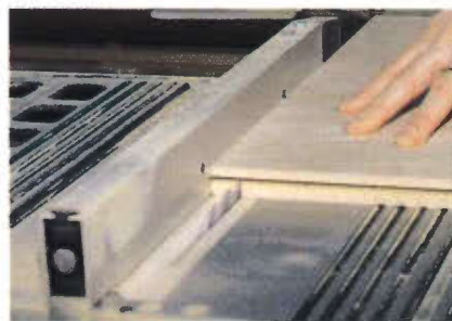
Photo 5 After adjusting the fence and blade height, the rabbet is completed running the panel flat on the saw table.
