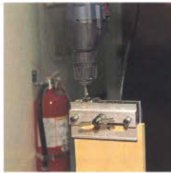
Photo 8 Using a doweling jig allows the dowel to be centered exactly. This reduces the chance of splitting in the particle board material.
