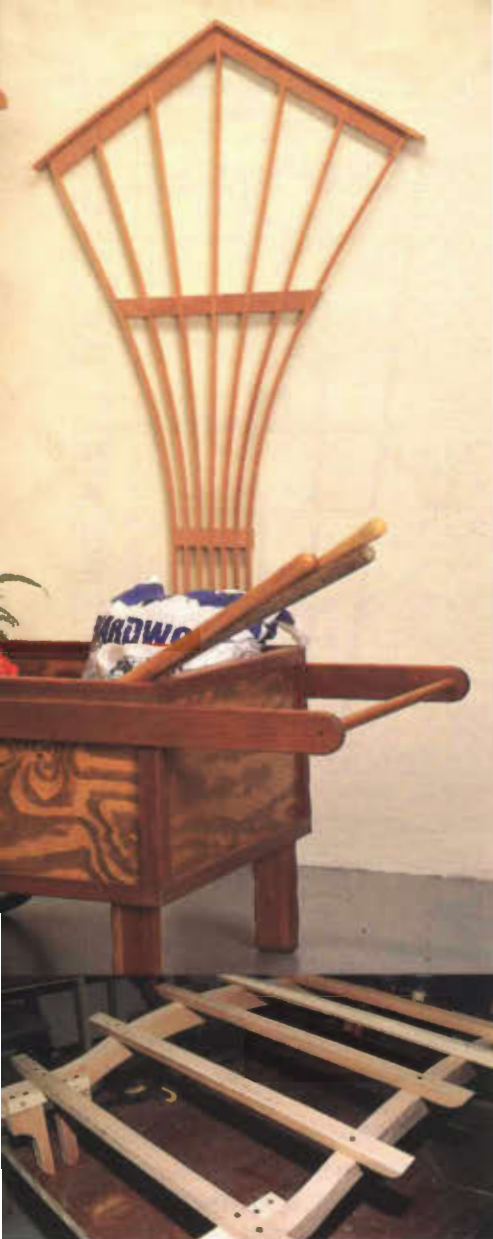
Photo 4 The ribs provide stability and a design element to the roof section.
