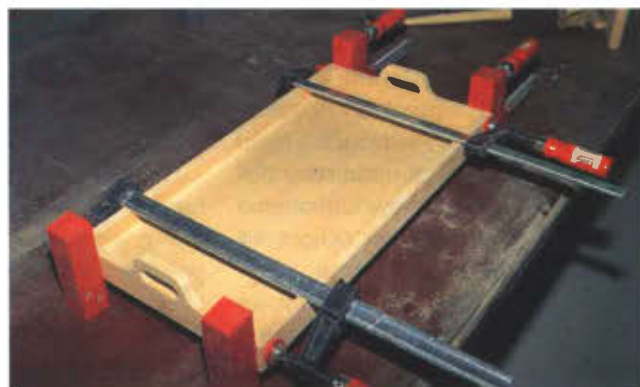
Photo 21 The tray is glued and clamped only on the miters to allow the bottom to float in the groove.
