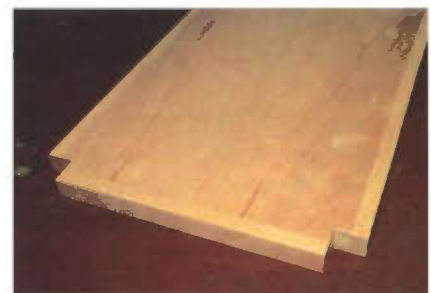
Photo 6 The corners on the bottom are notched at 1" to allow it to fit between the legs.
