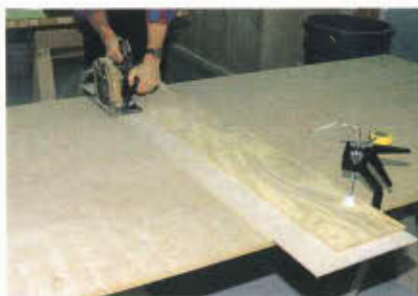
Photo 1 Building the mobile work station begins by chopping the big sheets to manageable sizes with the straight edge jig.
