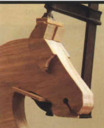
Photo 2 Dowels may be used when attaching the ears to strengthen them.
