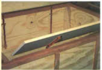
Photo 13 Copper tubing provides support for the optional "wings."
