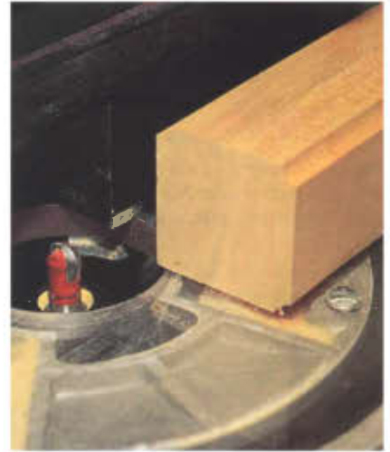
Photo 3 The cove bit used in a router table provides a simple but attractive detail on the legs.
