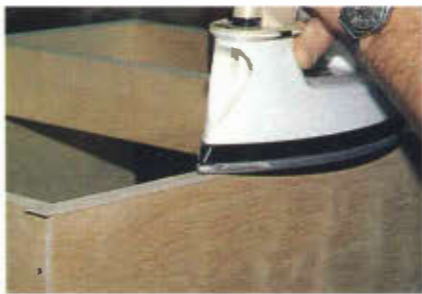
Photo 7 After assembly, the front edges of the cabinet are finished with veneer that has hot melt glue applied to the back side.
