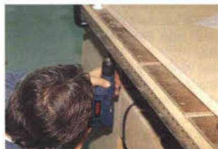
Photo 14 The continuous hinge for the folding top was first attached to the fixed top.
