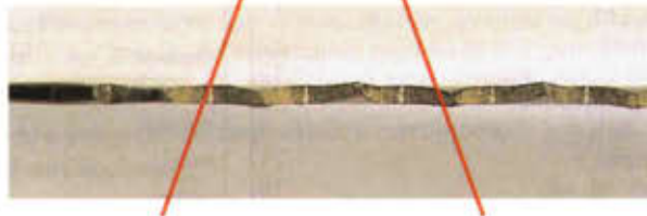
Crosscut teeth filed at a 70 degree angle
