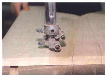
3 Before sawing the chair arm shape, make relief cuts.
