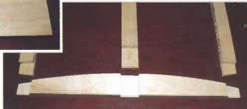
4 The frames will stay flat by clamping them together using a simple MDF backing board.
