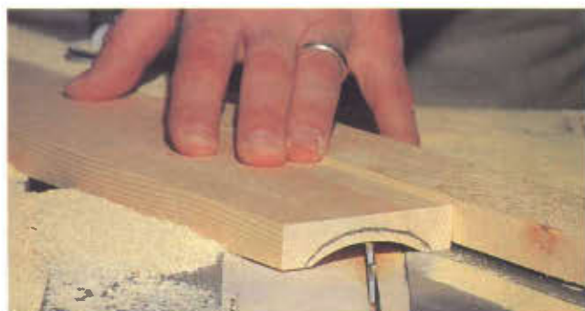
6 The coved crown mould is made using the table saw. Run the stock over the blade at an angle against an auxiliary fence set about 33 degrees askew to the fence.
