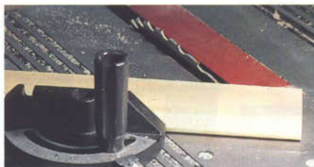
9 The compound miters for the crown mould are cut on the table saw by tilting the blade to 30 degrees and setting the miter gauge to 35 degrees.
