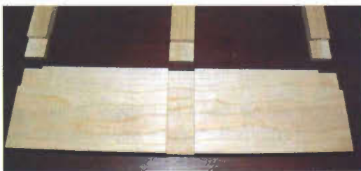
2 The end joints in the rail were made with a chisel, while the center was made on the saw.
