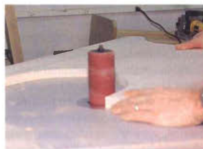
5 Sand the saw cuts smooth, working to the pencil line.
