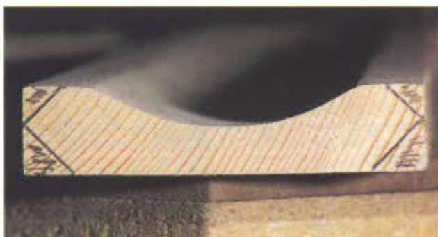
7 Complete the crown mould profile by making four, 45-degree cuts on the corners of the stock.
