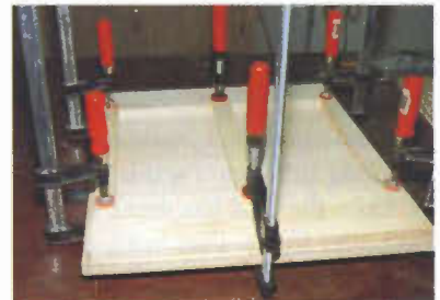
4 The frames will stay flat by clamping them together using a simple MDF backing board.
