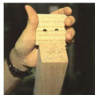
Photo 3 We used dowels to add extra strength to the cross-grain and end-grain glue joint.
