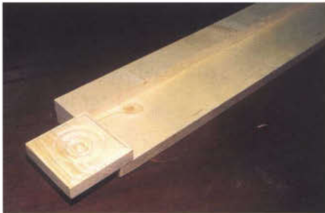
Photo 3 The rosettes overlap the facing board, and are set flush to the lower edge.
