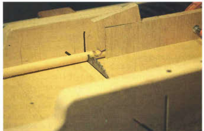
Photo 4 Use hold downs like the one shown here to keep your fingers away from the blade for cutting the short 1½"-long cross blocks.
