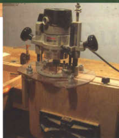
Photo 2 A jugged up mortising arrangement like this enables you to cut mortises quickly and accurately. This run of 160 mortises took about 27 seconds each, so I was able to complete the whole run in about 80 minutes.
