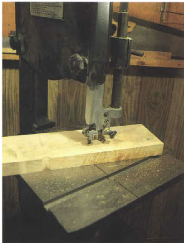
Photo 7 The arbor is simply a big isosceles triangle I cut out with a band saw and planed smooth.
