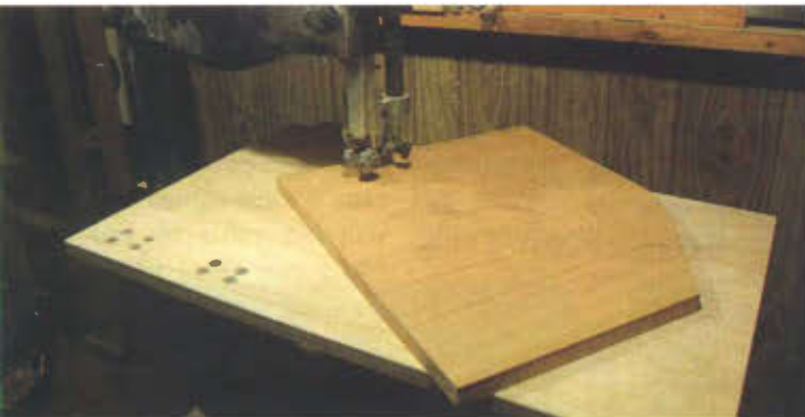
Photo 10 Once you've marked the center point on the bottom of the workpiece, drill a small hole about \frac{3}{8} "-deep into the underside of the workpiece and clip the projecting nail off so the workpiece rides flat and securely on the jig's surface. Then start the saw and advance the jig/workpiece assembly until the blade is located right on the centerline of the jig. Clamp the jig in place and rotate the workpiece until the circular top is completely cut.
