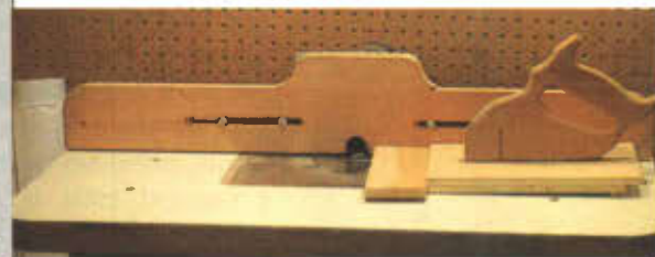
Photo 5 I used a push stick whose leading edge was cut at 3° to follow the workpiece as the tenon was routed. In this fashion I minimized tear out and managed to hold the workpiece firmly against the fence. It's safer, too.
