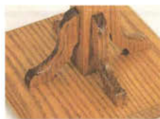
Photo 1 This detail shows the shape and attachment of the braces and the bevel on the base and feet.
