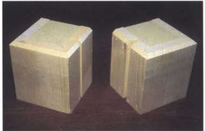
Photo 4 The assembled plinth blocks will be left and right, determined by the location of the groove cuts.
