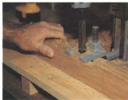
Photo 1 A bench-top mortiser makes the repetitive work more manageable.
