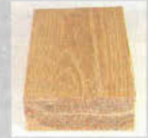
Flat cut wood has less than 45 degree end grain.
