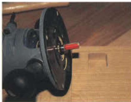
Photo 12 A flush cutting knife makes clean work of the through mortise in the arm.
