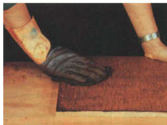
Photo 8 Applying wax with #0000 steel wool.
