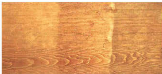
To reduce or eliminate blotching in a wood like pine, use a gel stain (left), or fill the pores with a stain controller before applying a liquid stain (right). The center has been left untreated.
