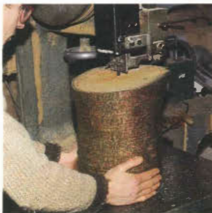
3 Cut the wood into two bowl blanks. This holly was stored on the ground, in the rain, for six weeks after being cut down.
