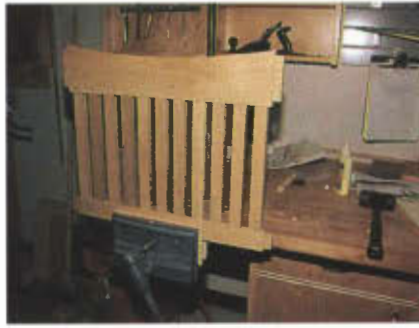
Photo 6 The side assemblies should fit snugly, but if you force them you'll split wood!
