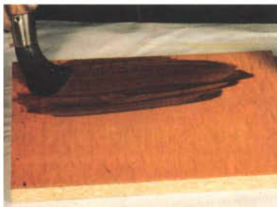
Photo 6 Applying glaze with a stiff bristle brush.
