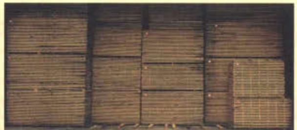
Commercial mills use large kilns to dry lumber steadily, but more rapidly than air drying. Note the stickers separating the stacks of lumber.
