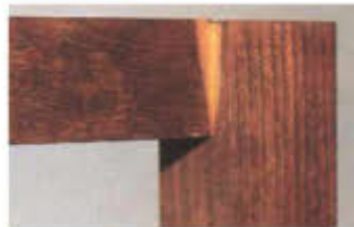
Seeped glue seals the wood pores, preventing stain penetration. You must remove this glue to get an even stain color.
