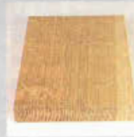
Quarter-sawn oak has near vertical end grain.
