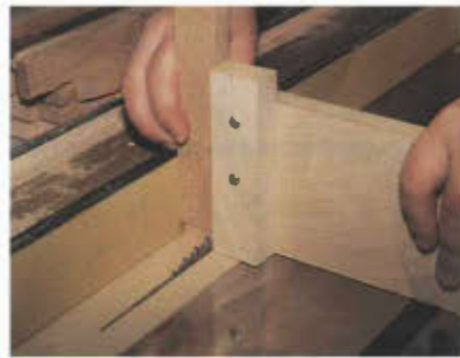
Photo 4 A simple setup on the miter gauge makes cutting the tenons more consistent.
