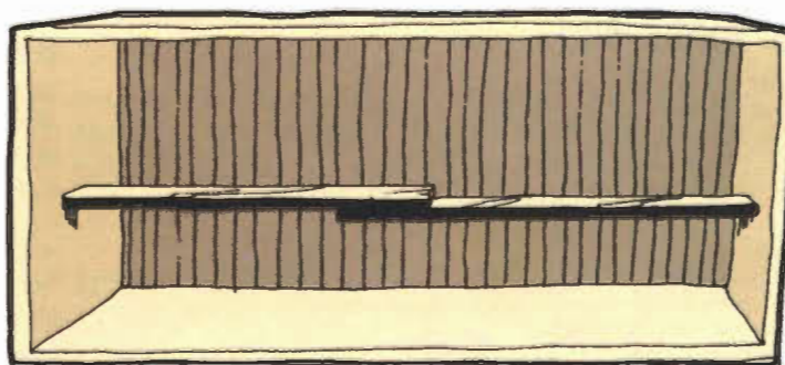
Diagram 1a: Pinch Rods Obtaining an interior dimension.
