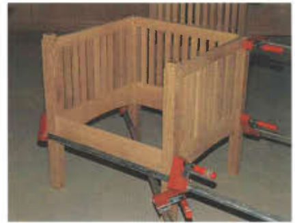
Photo 10 By clamping diagonally across the chair frame, square can be adjusted to perfect.
