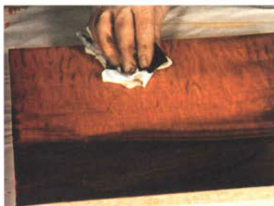
Photo 7 Wiping off the glaze.
