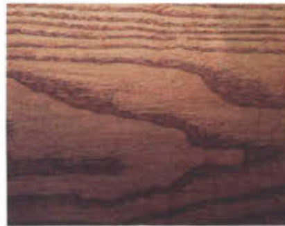
To more clearly illustrate sanding abrasion left behind, we sanded the above piece of ash with an orbital sander and 60 grit open coat paper. The deep spirals resulted from a worn-out pad on the sander.
