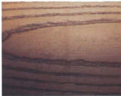
White ash prepared using an orbital sander. The right side has been sanded to 150 grit and the left side to 120 grit. The light stain highlights sanding marks that look like long spirals. The random orbit sander would break up this pattern.
