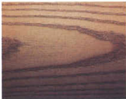
White ash prepared using a random orbit sander. A light stain was applied to show sanding marks left behind. The left side was sanded to 120 grit and the right side to 150 grit.
