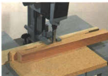
Photo 5 Side mortises are accomplished by placing a strip of wood between the work and the fence. The chisel cuts into both pieces. The extra-wide fence is a wood facing that is attached to the regular fence. Holes in the fence provide for the addition.
