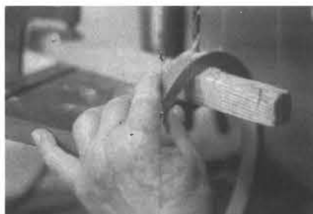
Photo 3 Mark opposite sides of the ring where the grain in either center ply or in solid stock runs tangentially. Drill \frac{1}{4} " holes for the pivot bolts.
