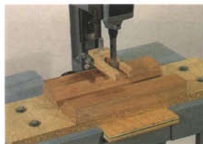
Photo 6 The V-block jig set up on the benchtop.
