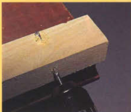
Photos A, B, & C One way to cut the pocket is to drill the screwhole first, marking where the drill bit emerges from the wood. (Make sure you know which face will show, and drill through the opposite side.) Then use a chisel to pare away the pocket.
