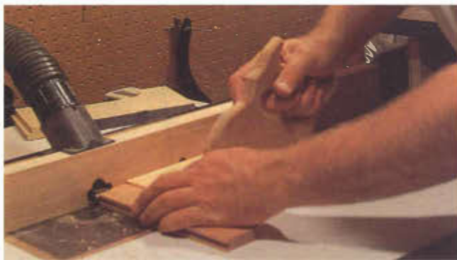
Photo 8 Cut the tongues for the rails of the door by routing them against a fence on a router table. The push stick helps keep it square to the fence.
