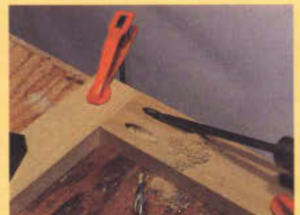
Photos E & F Commercially available jigs make quick work of pocket joints when producing them in quantities of ten or more.
