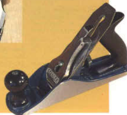
Photo 13 The bench plane is used for finesse work, like removing a see-through shaving, and for cruder jobs, like smoothing a rough board.
