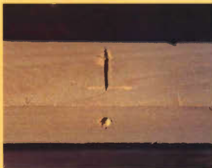
Photos A, B, & C One way to cut the pocket is to drill the screwhole first, marking where the drill bit emerges from the wood. (Make sure you know which face will show, and drill through the opposite side.) Then use a chisel to pare away the pocket.
