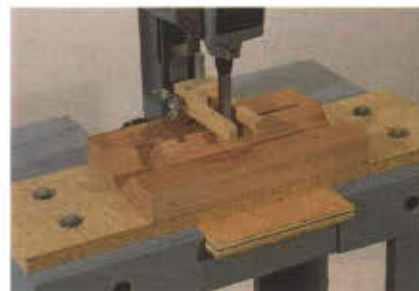
Photo 9 Mortising into the corner of square stock is also feasible. Start the cut very slowly to avoid allowing the bit to wander off the corner.
