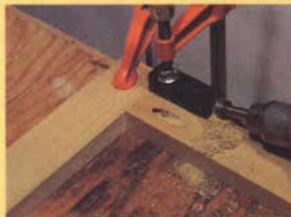
Photos E & F Commercially available jigs make quick work of pocket joints when producing them in quantities of ten or more.
