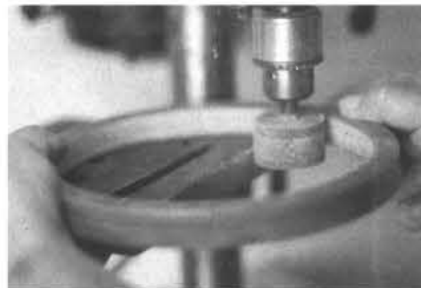
Photo 2 With a drum sander on the drill press, sand the inside of the ring until smooth. Then apply French polish by hand to this surface.
