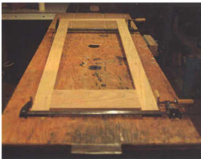
Photo 5 Assemble the jelly cupboard face frame, making sure you clamp it square. Check for square by measuring diagonally across inside corners. The measurements should be exactly the same. Reposition the clamps if they're not square. Be fussy with this, as an out-of-square cabinet is more useless than yesterday's lottery ticket.
