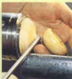
G Keep shaping the knob until the lid drops into your hand. Oak isn't ideal for boxes because it can split at this point.
