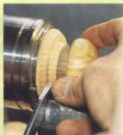
H If you want to finish off the lid perfectly, turn a jam chuck from the waste and remount the lid, then finish the knob.
