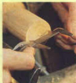
I Mark out the hole in the body by subtracting 3/16" from the inside lid diameter, with the caliper points down.
