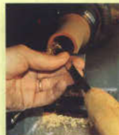
J Hollow out the body with the method you prefer. I used a bedan in this particular case.
