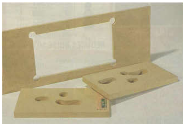
3 The templates and frames are made from medium density fiberboard (MDF). The shape of the slots in the templates is formed by a computer controlled machine. Diamond-tipped bits perform the cutting.
