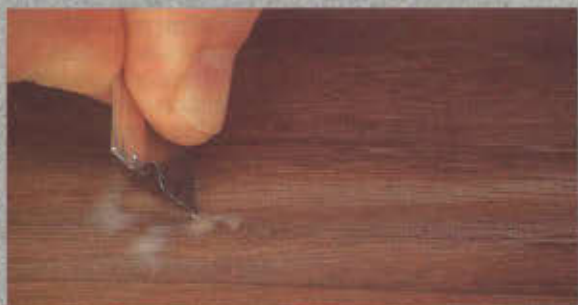
Here I'm removing a glue stain from a piece of walnut using water and a razor blade.
