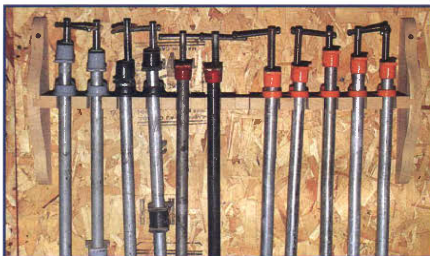
5 This is the same design for the bar clamps that has been adapted to hold pipe clamps. It's always a good idea to build these racks a little bigger than you need them. (You never know when you might get another clamp for your birthday.)
