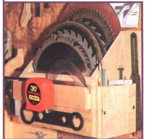
9 With a little imagination, you can turn this blade keeper into a virtual table saw "tool belt."
