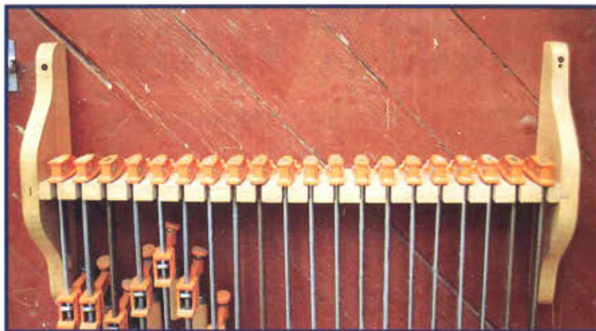
4 Build this simple rack for your bar clamps so they don't get tangled in the corner of your shop.
