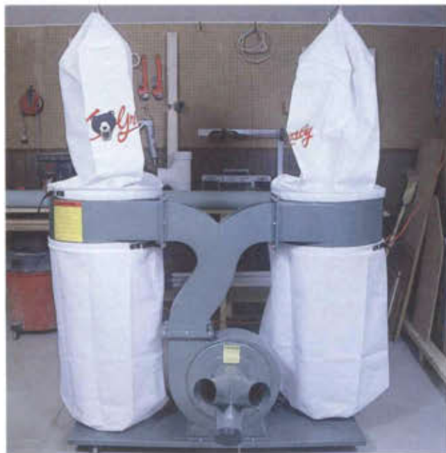
A meeting of the Klan? Casper meets Banquo's ghost? I think not. This is the three-horsepower, four-bag dust collector from Grizzly.
