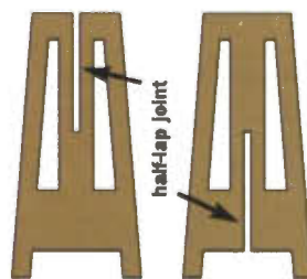
STEP SIX: Lay out the location for the poplar cleats that hold the triangular braces. Taller people will be comfortable with the braces about 6" off the floor. Shorter folks will like the braces higher. If you raise the braces, you
