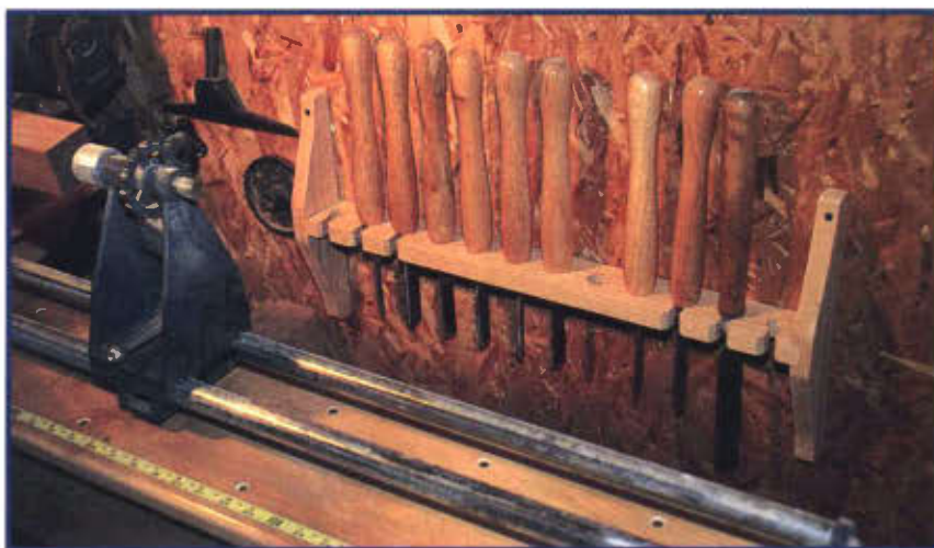
6 If you're tired of scrounging around for your lathe tools, this rack mounts easily behind your lathe, giving you quick access to the correct tool.
