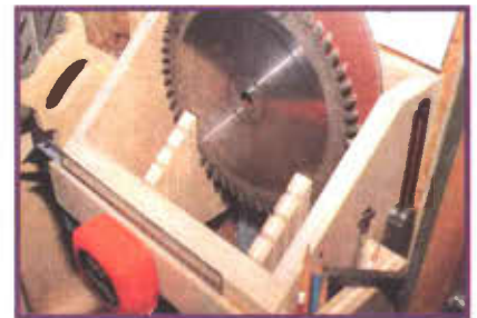
8 This saw blade rack keeps your blade collection handy by your table saw, protects the tips of the blades and can even store many of the other tools frequently used at the table saw.
