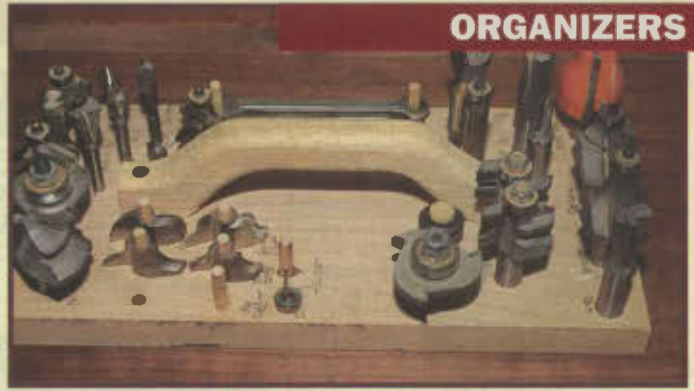
7 This router bit caddy protects the cutting edges from banging into each other and into your fingers.
