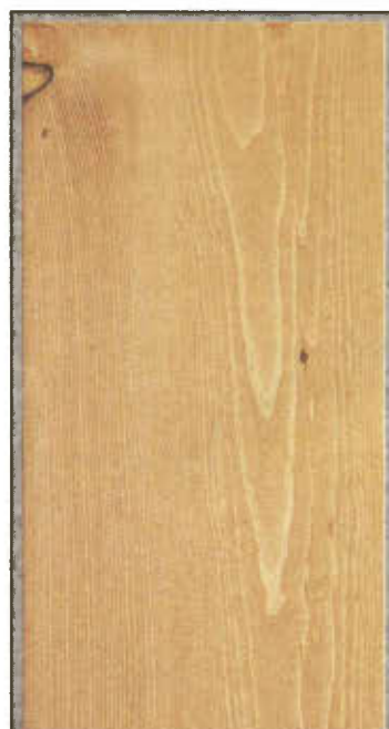
Pine wash coated with shellac then stained with Minwax cherry.
