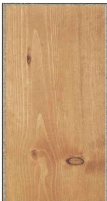
Pine with Minwax cherry applied directly to wood.
