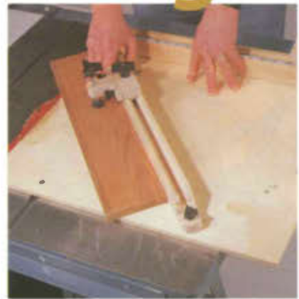
Make miter cuts with this sure-grip hold-down...
