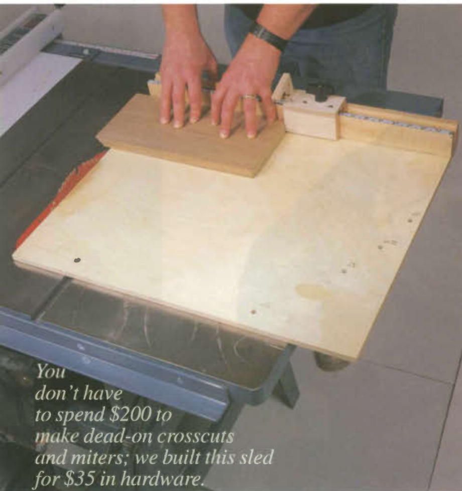
Make miter cuts with this sure-grip hold-down...
