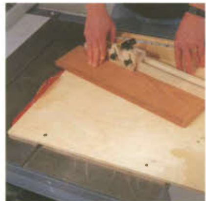
... or use the attachable featherboard for repeat cuts.
