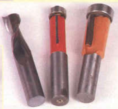
Above left is an upcut spiral bit, which is excellent for removing waste in mortise operations; center is a straight flush cutting bit; and on the right is a shearing flush cut bit for cleaner, easier operations with dense or highly figured woods.
