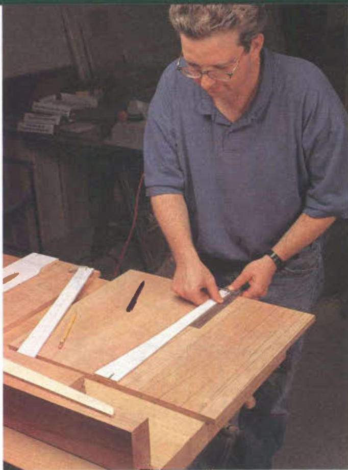
The templates for the slats are provided on the scaled-down grids. After enlarging them, lay out the templates on your wood, cut the tenons on the end of the board and band saw the slats to shape.
