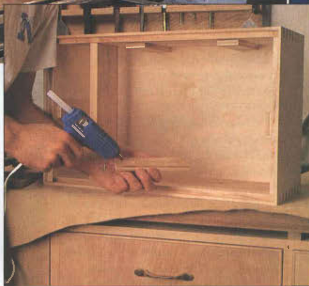
Use hot melt glue to attach 6"-long blocks that keep the saw kerf open when you cut the front off the cabinet (inset). After that, ripping the cabinet is almost cake.
