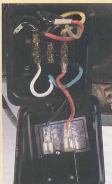
Here's the box on the motor for our Jet table saw. You simply move a couple leads and your saw is then ready to take 240 — as soon as you change the plug, that is.
