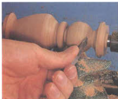
After the top is complete, the blank will be parted in two and each half will be remounted to bore the hole for the glass vial.
