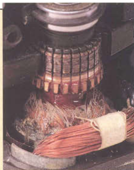
Assembled armatures and commutators at Makita's plant in Georgia. We were impressed with the rigorous tests Makita performed on their universal motors.
