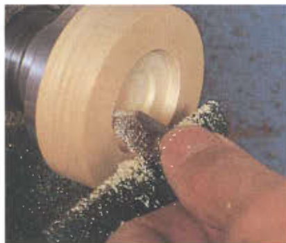
Turning a pocket in the wooden auxiliary faceplate to accept the tenon on the end of the perfume vial blank.
