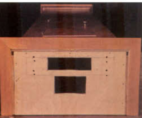
Here you can see the cutouts to accommodate the swinging pendulum and the hanging chains from the works.
