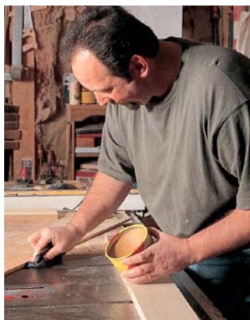
After years of doing this, I've found that a little furniture wax makes this cut a lot easier.
