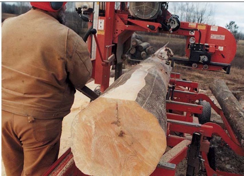
Here a portable band saw mill cuts into a log of red oak that was on the bottom of a lake for 100 years or more.
