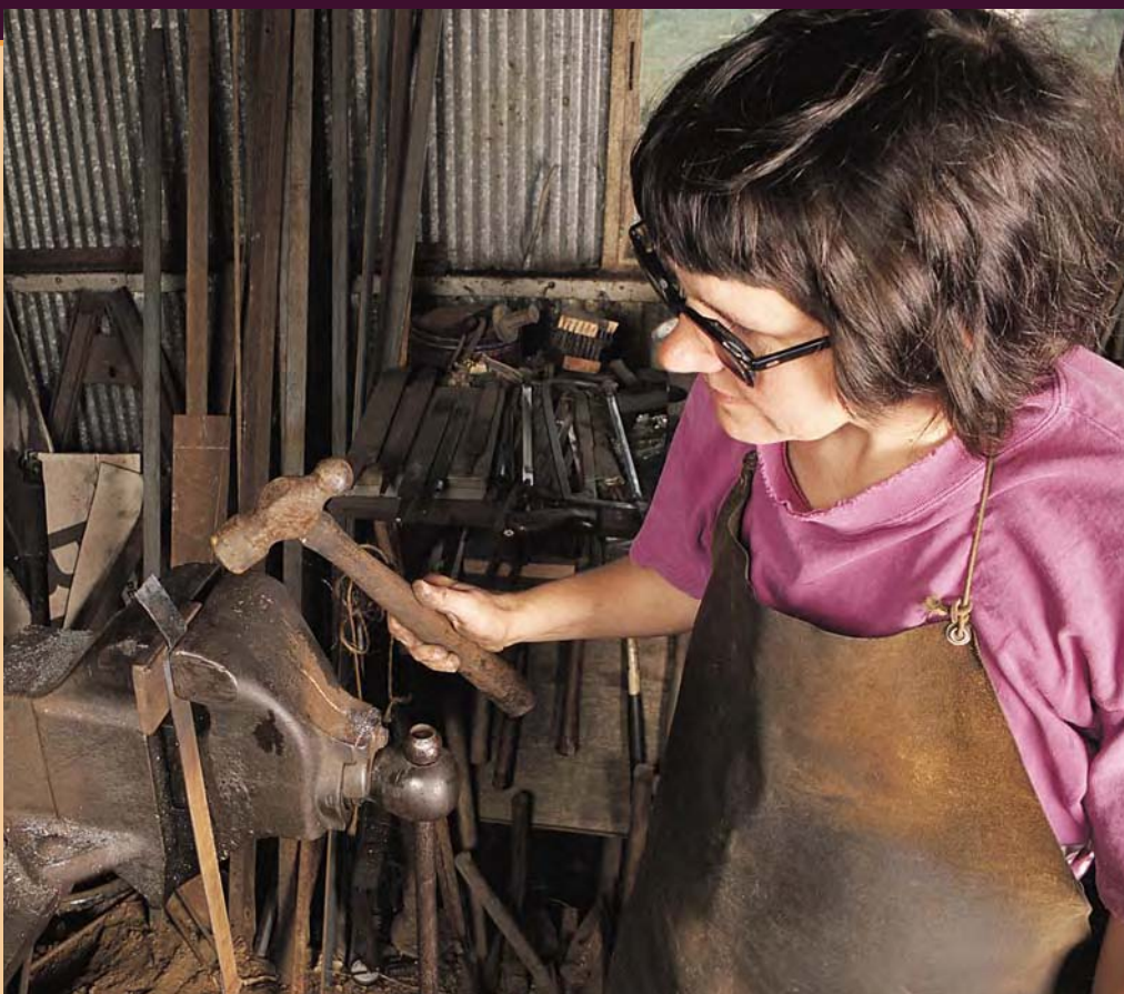
Accomplished blacksmith Marsha Nelson starts the process of hand making a hinge by cold bending flat stock on a jig secured in a vise. The jig provides the correct opening size for the the pintle, or hinge pin (above).
