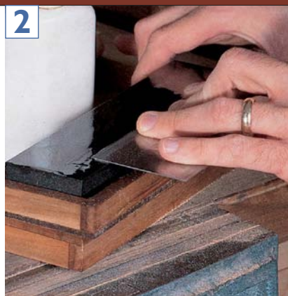
Remove any burrs you created when filing the scraper by placing the tool face down on a sharpening stone and rubbing in a circular motion.
