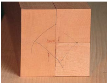
The diamond marked on the tops of the four legs will always allow you to recognize the inside and outside faces of the legs.
