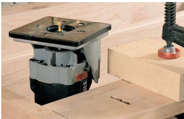
A keyhole bit fitted in a hand-held router and run along a guide block is an easy way to attach the shelf to a wall
