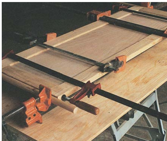
The lid is a simple frame-and-panel assembled with biscuits and glue. But because the panel is a piece of plywood, you don't need to worry about seasonal expansion or contraction.
