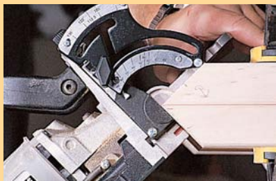
Or, if you have a fixed 90° fence on your tool, you can clamp them together this way to cut your slots.
