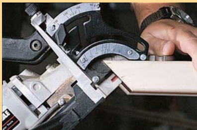
The fence on the Porter-Cable 557 allows you to biscuit your miters with the fence on the outside of the joint — a nice feature.
