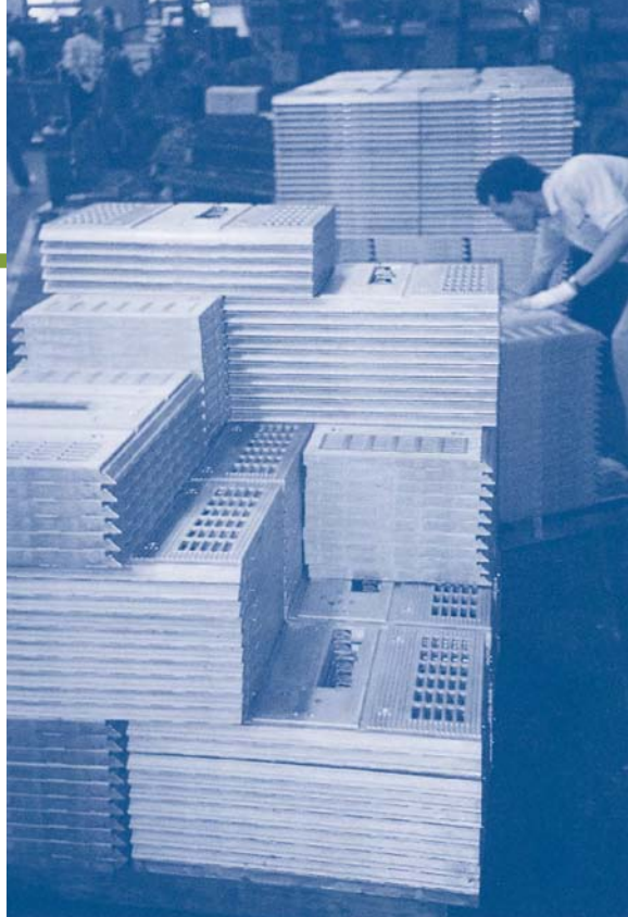
At Hsum Tsao, a Taichung aluminum die cast molding plant, a worker knocks off excess aluminum from a miter saw fence casting (left). Castings for benchtop saws are stacked for machining and assembly later (right).
