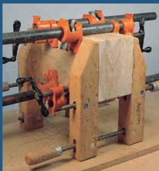
This block isn't going to fall apart! It pays to be generous with the clamps, glue and the drying time.
