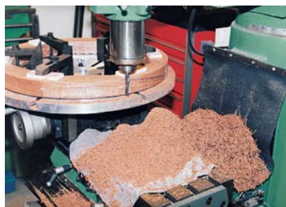
Milling machines excel at dealing with round shapes. Clockmakers will be amazed at what this machine could do for their woodworking.
