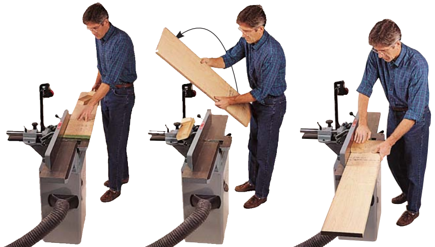
Face joint stock that's wider than your jointer capacity by removing the guard and setting the fence to a bit more than half the width of the board. Run one side as you would normally, taking light passes. Then flip the board end for end and face joint the other side. Take a couple passes on each side before turning and be careful not to get too deep a ridge in the middle.
