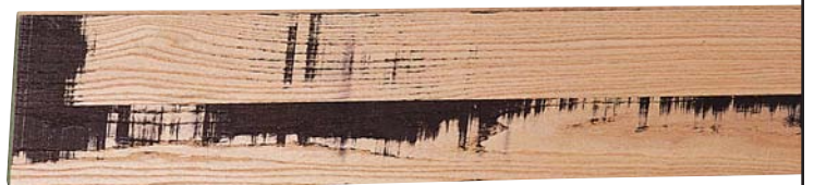
After several passes on each side of this face, the board is about ready to run through the planer.
