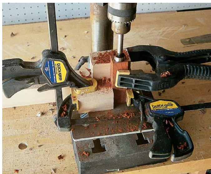
When drilling into end grain, you can't use too many clamps. The stop also ensures that the small piece is perpendicular to the table.
