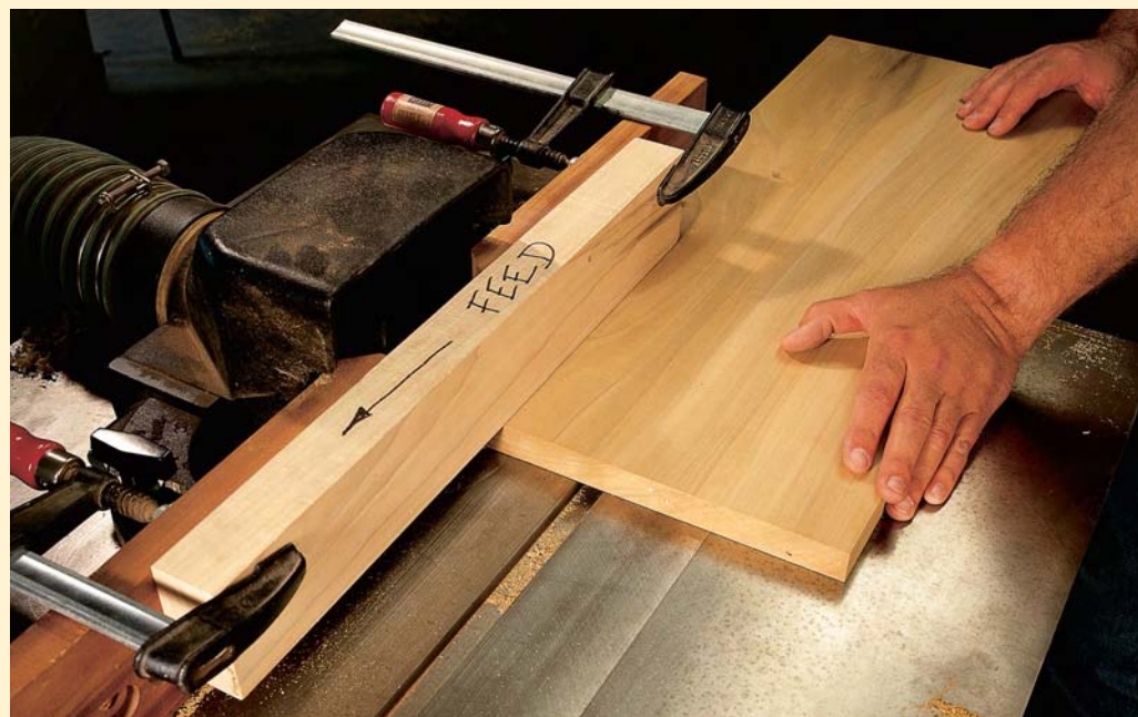
Using the right guard and keeping your hands away from the cutterhead will help avoid accidents.
