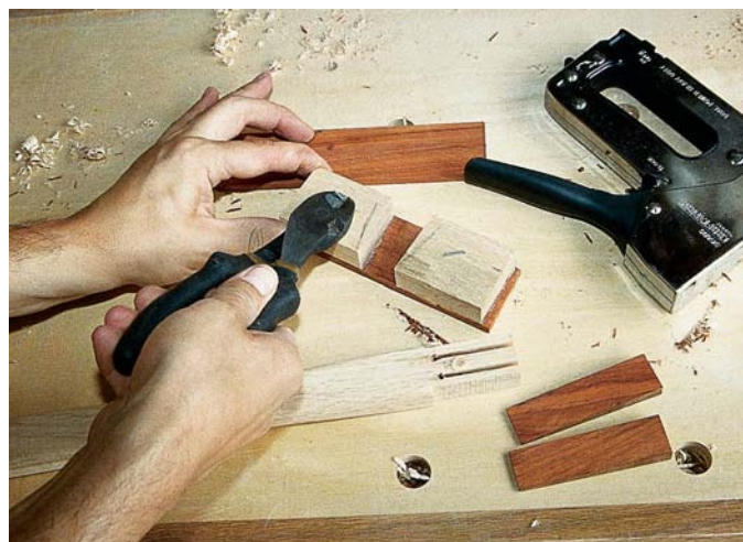
Clip the heads off of staples to prevent the laminations from slipping during glue-up.
