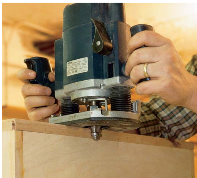
Go slowly while rounding over the edges, as the cherry can tear out and splinter if a cut is rushed. The roundover is key to the smooth, clean feel of the piece.
