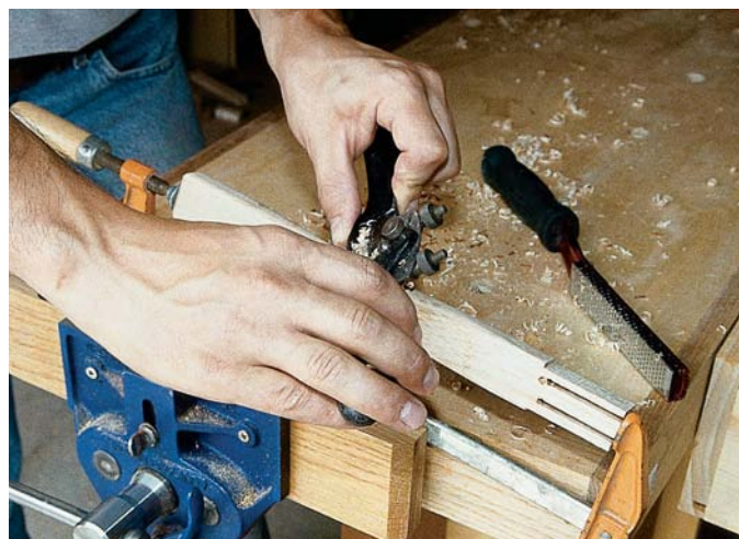
You can shape the handle with a spokeshave in less time than it takes to read this article. By clamping the handle as shown, you can spin the handle to quickly round over all four edges.
