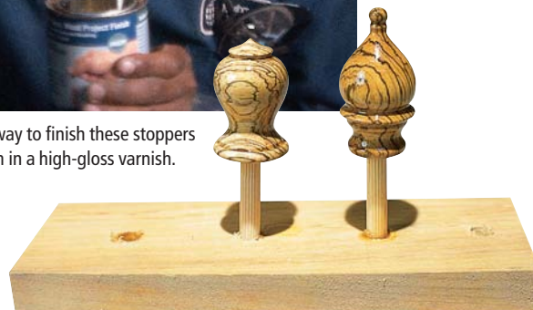
After applying the finish to the stoppers, the best way to let them dry is to make a small rack that holds the stoppers' mounting dowels.
