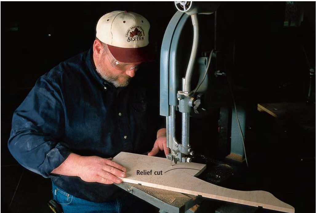
Notice the relief cut I made in the sides. By removing the waste in smaller hunks (instead of all at once), the blade is more maneuverable.
