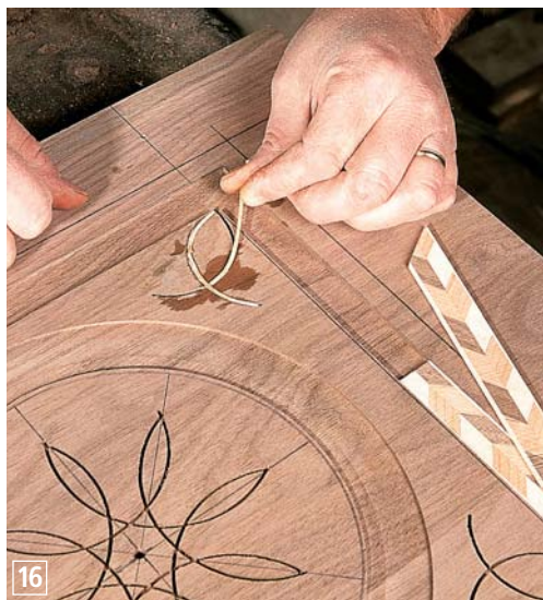
16 To make the banding for the corner arcs, set your table saw to once again slice 1/16" strips from a larger piece. Then carefully slice the strip to a little over 1/8" thick. A straight edge and utility knife will serve well here. Then add a little glue and press them into the recess. Make some extra strips in case some snap. I used tiger maple, which is pretty brittle. Holly would have been easier to work with.
