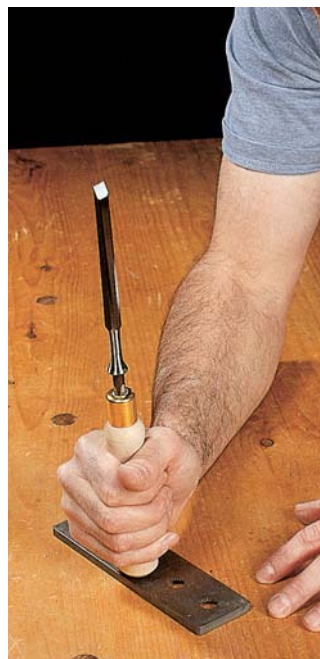
Seat the tang in the handle by repeatedly striking the end of the handle against an iron plate or machine table.
