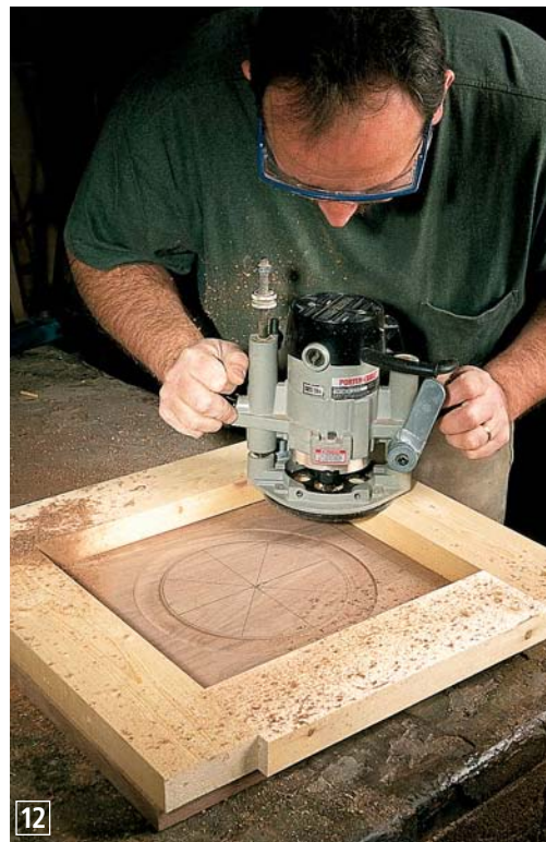
12 For the next step I chose to make a simple 2x4 frame and used a bit with a top-mounted bearing to create the outer border recess. This ensures that the corners will meet accurately. I used a 3/4"-wide straight bit to make the cut with a single pass. After the cut, use a chisel to square out the corners.
