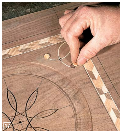
17 For the "berry" designs, I used a 3/8" plug cutter to make a number of 1/8"-thick dots. Carefully glue these in place. The berries in the center of the pattern are created in the same way.
