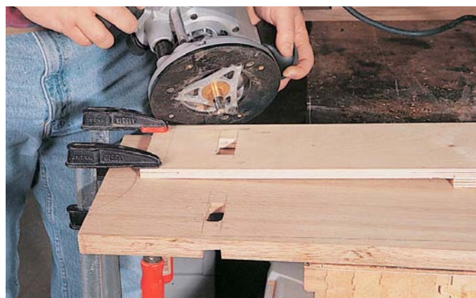
This simple scrap-wood jig made angled mortises a fairly simple task.
