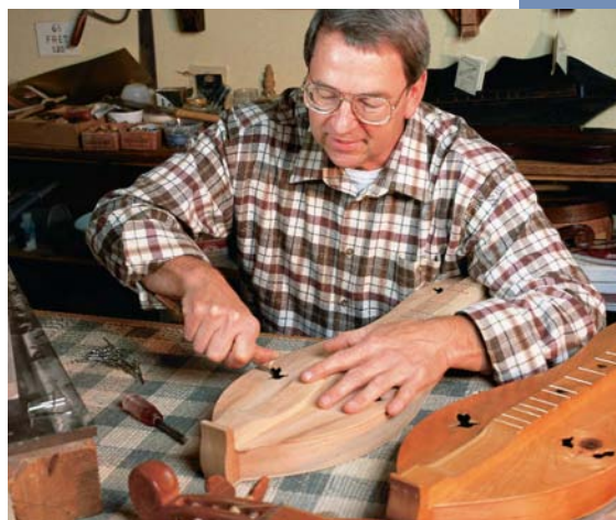
May's clamping jig is a set of \frac{5}{16} " bolts that are held in a special pattern frame. There are multiple dulcimer profiles and each requires a matching "spring clamping jig." All bolts are spaced properly to place just the right amount of pressure at exactly the right spot. While one jig costs about $30 to make, it replaces about 40 spring clamps and makes a better product.
