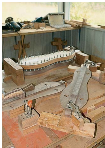
May's clamping jig is a set of \frac{5}{16} " bolts that are held in a special pattern frame. There are multiple dulcimer profiles and each requires a matching "spring clamping jig." All bolts are spaced properly to place just the right amount of pressure at exactly the right spot. While one jig costs about $30 to make, it replaces about 40 spring clamps and makes a better product.
