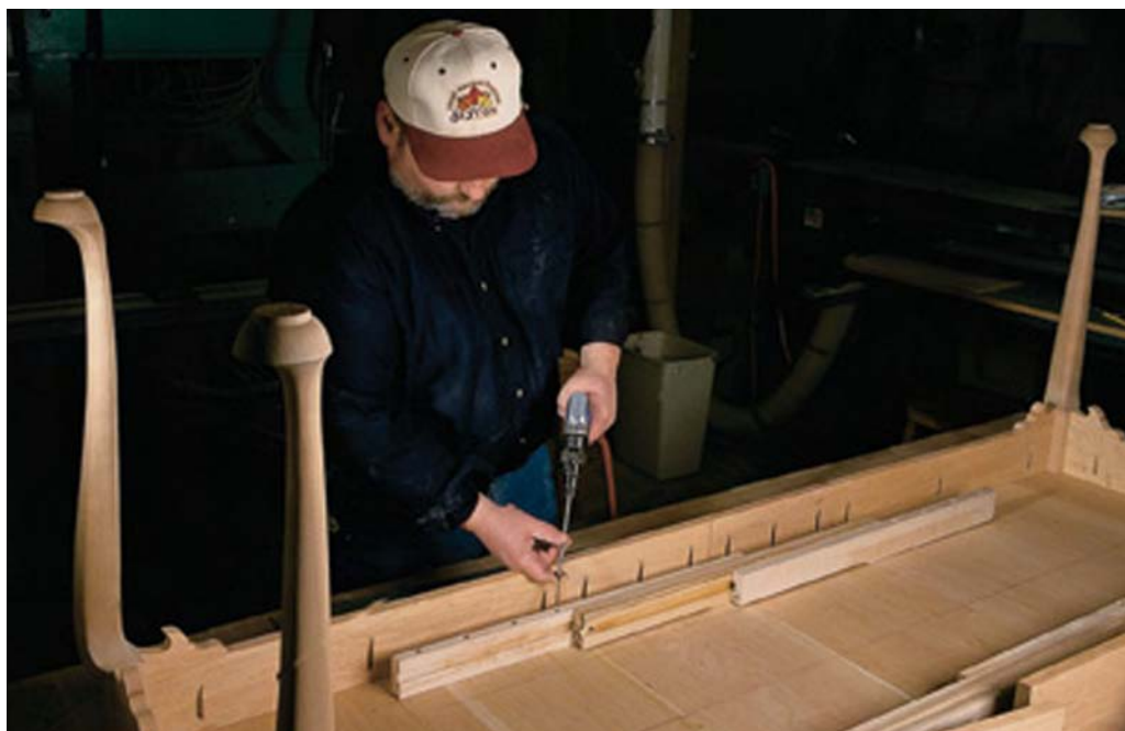
Make sure your table slides are not fully extended when you screw them down. Otherwise, you'll be in for a rude shock: You won't be able to get your leaves out.
