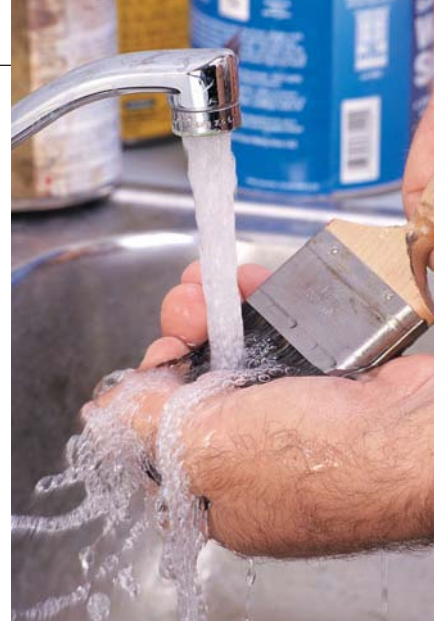
The final step in cleaning any stain or finish out of a brush is to wash it in soap and water until suds form easily. That's when you know your brush is clean.
