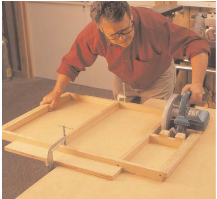
I use this jig as a saw base as much as I use it as table saw, especially when cutting up large sheet materials.
