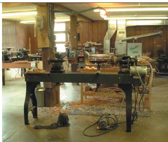
The ground floor work area features one of the classic Conover lathes. I also noted some Nova lathes. Eight-inch bench grinders help students master the art of quick and easy sharpening. The anti-fatigue mats make working on concrete much more comfortable. Ample windows and many banks of lights provide great illumination that leads to less eye strain and better work.
