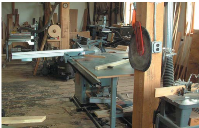
The Unisaw in the prep area has a crosscut sled and, when needed, a traditional Unifence. The saw is on a mobile base so students can move it to work with longer or wider work pieces. A drum sander offers an affordable way to surface even highly figured woods such as curly maple. Notice that the central dust-collection piping is carefully tucked in out-of-the-way places for efficient use.
