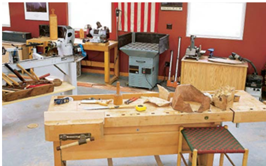
The single most important tool in my shop is the 352-pound European-style Ulmia workbench. This heavy-duty bench can't be pushed around and is like an aircraft carrier with lots of room to do whatever I want. It also has a tilting drawer which (confession is good for the soul) is one great catch-all with a lock. The drawers never stay neatly arranged if much work is getting done in the shop. I prefer to keep the bench pulled away from the wall so I can work on all sides of it as necessary.
