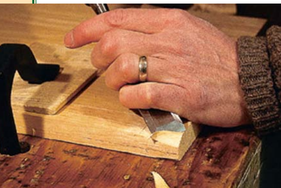
Before raising your bottom panel's cross grain, chisel down the corners so you won't split the off the edge as you plane.
