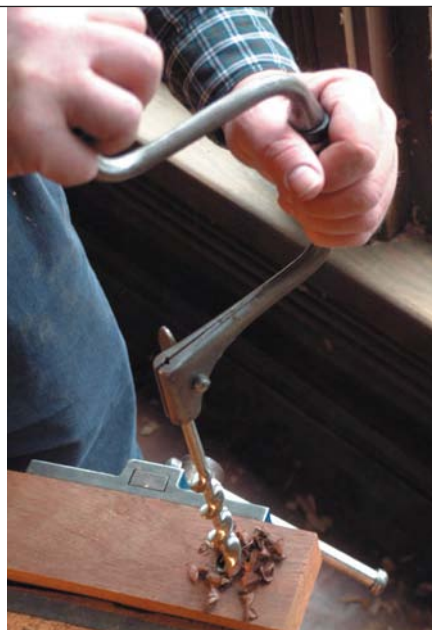
The brace and bit produces immense amounts of torque that your cordless drill could only dream about. Plus, many models (not the one shown here) have a ratcheting feature that allows them to be used in corners and right up against wall moulding.
