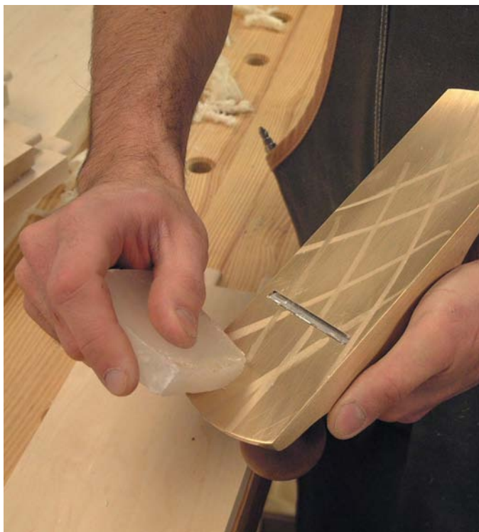
A little canning wax on your sole makes the work easier and your cuts lighter.
