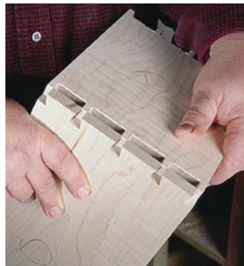
The WoodRat allows me to space the pins and tails in almost any configuration I please. And because one part acts as the template for the other, the fit is nice and firm.
