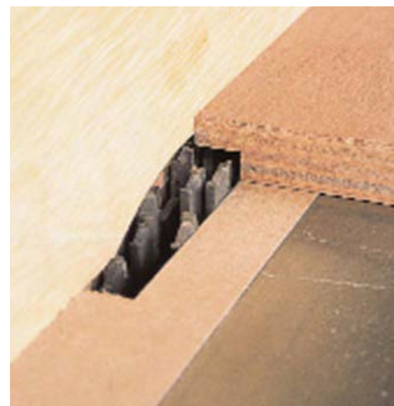
Clamp a sacrificial facing – a strip of luan plywood here – to your table saw fence when cutting rabbets with a dado head. Run the cutter up into the facing, exposing only enough of the cutter to form the rabbet.
