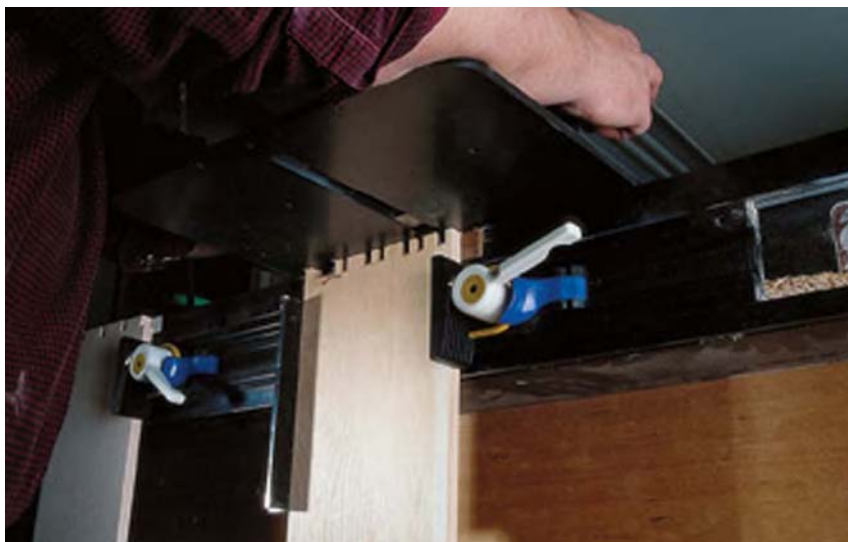
The WoodRat in action – as seen from below. Check out the company's web site at woodrat.com to see all the useful joints this system can build.
