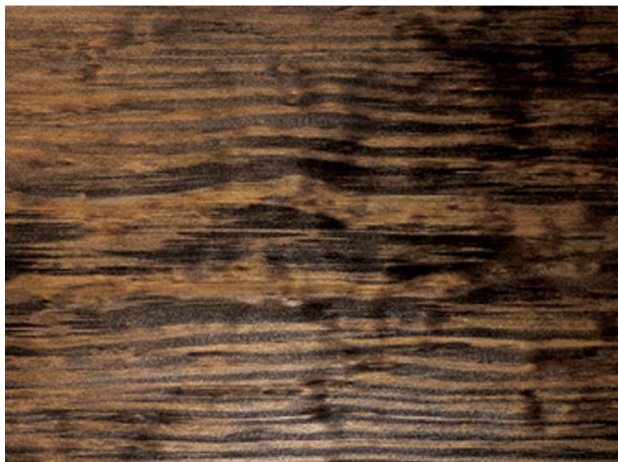
Pine is notorious for the uneven way it takes stain. Here we hand-planed a board of Southern yellow pine to perfect shimmering flatness and applied a walnut stain. This board experienced both grain reversal and significant blotching. In other words, the problems occur with even the most careful preparation.
