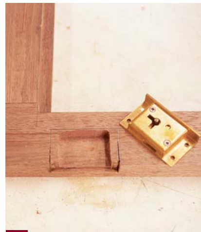
15 Install the lock into your door, then fit both doors into place and install the hinges, making sure to allow equal spacing around the doors.
