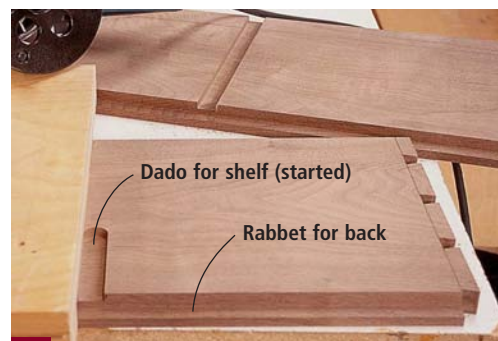
2 With your dovetail joints complete, cut the \frac{1}{2} " x \frac{1}{2} " rabbet for the backboards, then locate and create the \frac{1}{4} "-deep x \frac{3}{4} "-wide dado for the shelf. Once you have these complete, you should be able to assemble the dovetailed box.
