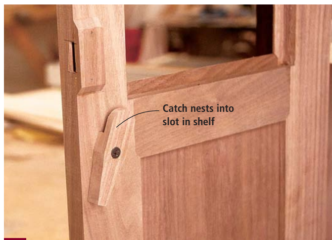
17 Using a biscuit joiner, make a groove in the bottom edge of the shelf, just behind the stile and 1/4" from the shelf front, to accept the door catch. Next, mark the location of the lock strike and create a catch. It is also possible to purchase an angled strike plate from the lock supplier to eliminate this procedure.
