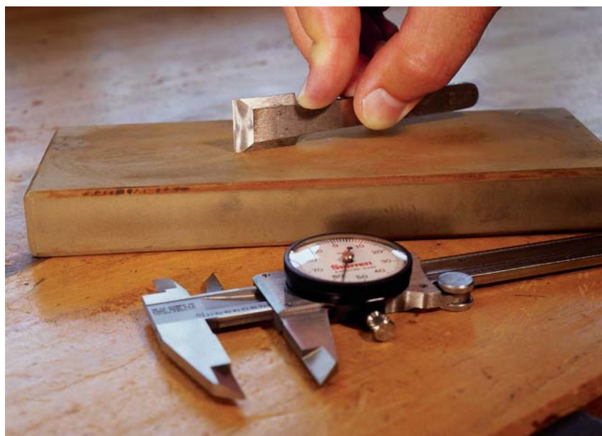
Your iron should be .006" to .010" wider than the sole. To get your iron to this width, carefully work the sides of the iron with a coarse bench stone. Check your progress with a dial caliper.
