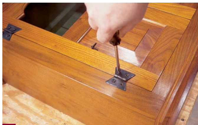
18 Install the glass. Reattach the hinges, reinstall the lock and apply a coat of paste wax. And with that, your cupboard is done.
