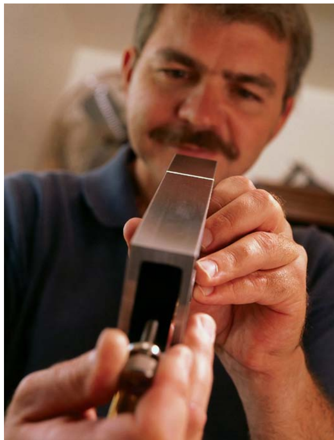
Once your iron is ready for cutting, install it in the plane and adjust it for a very light cut. Simply sight down the plane and slowly advance the iron until you can see just the edge.
