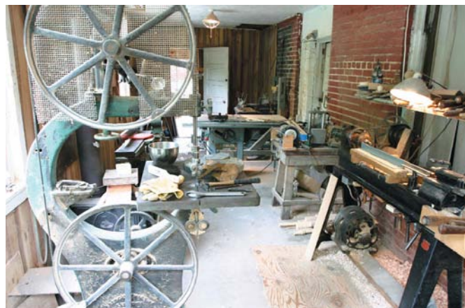
Weber is working on making a cover for his 1918 Crescent Manufacturing band saw. The heavy-gauge mesh wire you see here is part of that cover.
