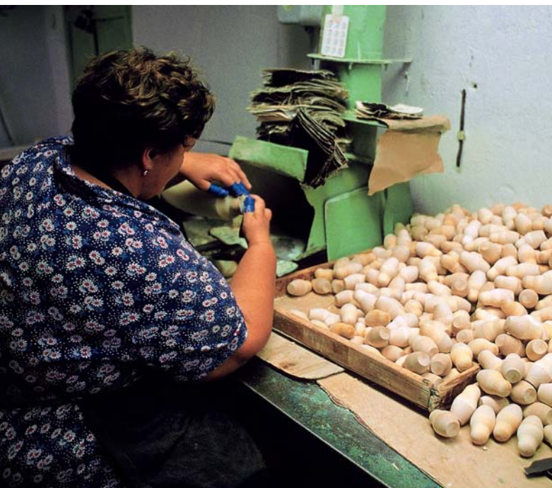
In the Nolinsk factory, a final sanding is done on a small spindle lathe. The operator protects her fingers with blue electrical tape.
