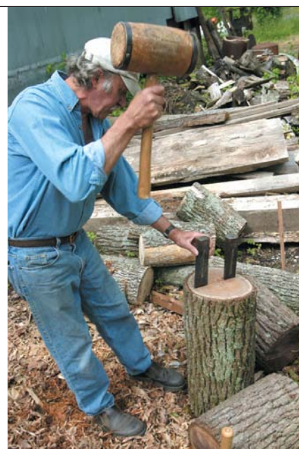
Weber splits a log outside his shop using an iron-bound mallet (called a beetle) and wedges.
