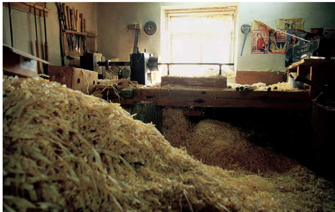
This is one of many backyard lathe sheds in Maidan. The lathe operator builds and maintains his own machinery and keeps his tools sharp. Sweeping the floor, however, is not a major consideration.
