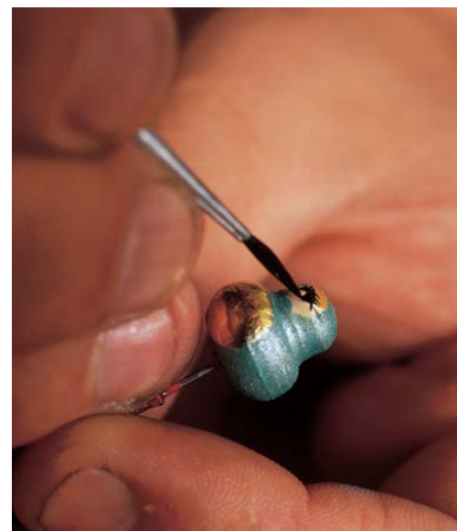
To paint “micro” matryoshki, paintbrush bristles are brought to a very fine point. To hold the small doll, the artist sticks it onto the end of a disposable syringe needle.
