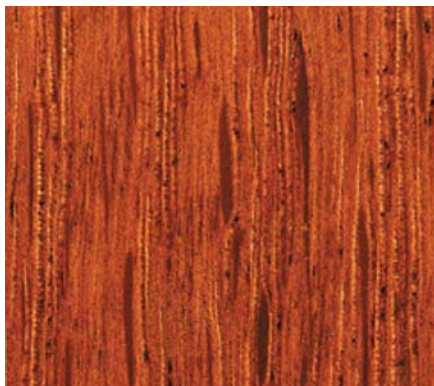
One of the disadvantages of a dye stain is that it doesn't get into the pores of open-grained wood, such as this piece of red oak.
