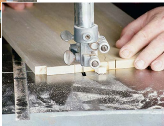
After I lay out the tails on the drawers' sides, I cut them out using my band saw.
