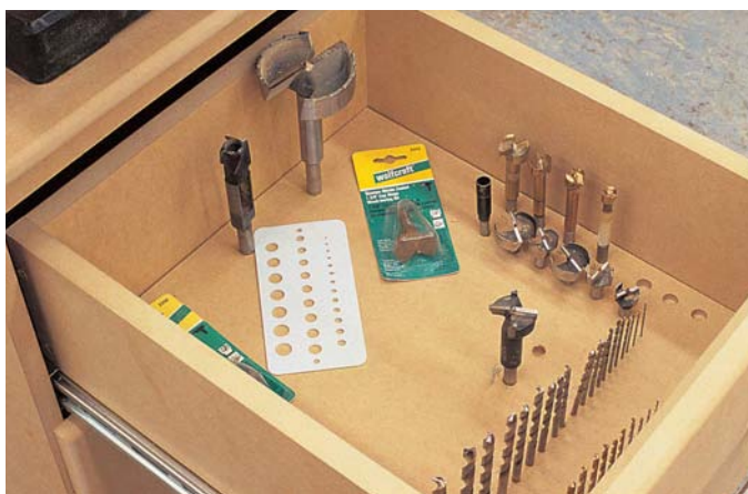
I store and index my drill bits in the top drawer by drilling holes in a piece of \frac{3}{4} "-thick MDF and sitting it in the drawer box. As my bit collection grows, I can always remove this platform and drill new holes.
