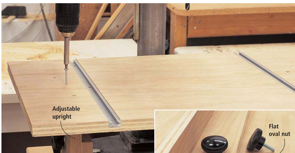
Attach the plywood table, with the tracks already installed, to the adjustable uprights with screws. Secure the fence to the T-tracks using knobs with a threaded shaft and flat oval nuts (right).
