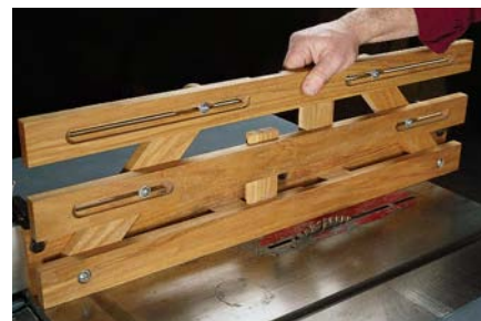
Just loosen the machine screws and the fence can be adjusted to any height.
