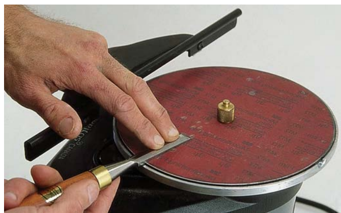
The Mk. II also allows you to flatten and polish the backside of your tools and remove the tool's burr on its backside while sharpening.
