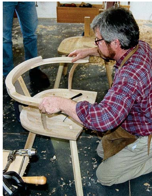
Fleming positions the bow on one of the drilling jigs and the “horns” of the chair, which are the curved spindles underneath the arms at the front.
