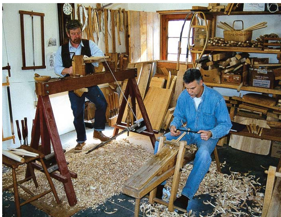
David Fleming turns a few spindles on the pole lathe as John Hoffman, the other student in the class, gets comfortable with the shaving horse and drawknife.
