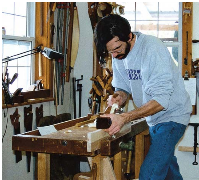
Here I'm shaping the crest rail before steam-bending. The crest began as chunk of ash, but after less than an hour of work it was a perfectly flat piece of wood with two straight edges.
