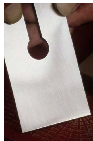
After this second movement, the scratches across the blade's width will be replaced with lengthwise scratches.
