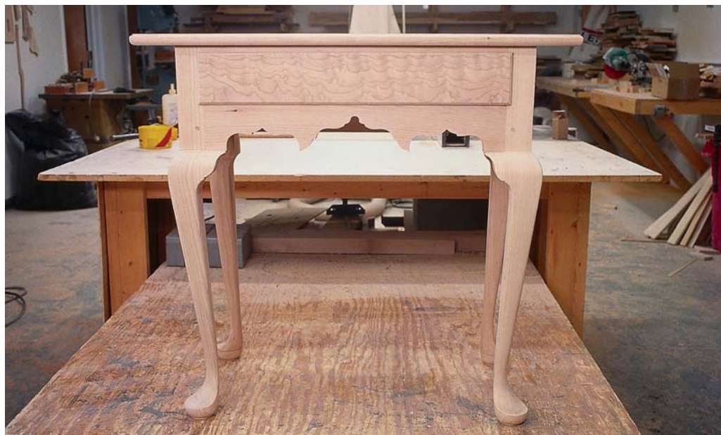
All the fitting and sanding have created a nice piece of furniture, but it still needs a replica finish. Don't try and short-circuit this last step. Even though the piece is sanded, in order to apply a water-based finish, first wipe down the entire piece with a wet rag, then sand again before applying the stain.
