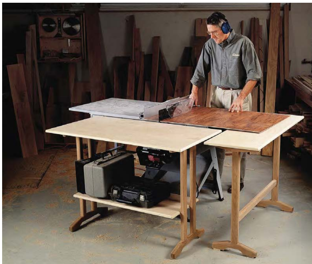
Outfeed support is critical to safe and accurate work. If your work cantilevers off the side, support it there, too.
