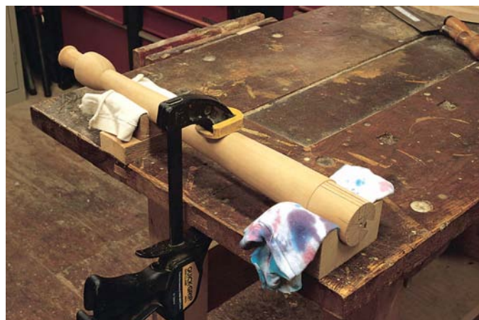
Fix the pedestal on your bench with a pair of U-blocks and a clamp.
