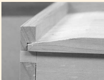
Traditional drawers used raised panels made of solid wood for the bottoms. These are easily made on a router table with a raised-panel bit, then fit into a standard groove in the drawer sides.
