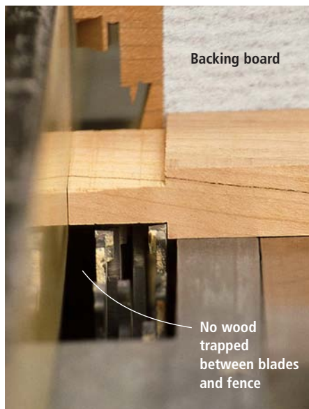
The second pass has the work against the fence and defines the face shoulder. Note there isn't any wood between the fence and blades, so the chance of kickback is minimal. The backing board reduces the chance of tear-out at the shoulders.
