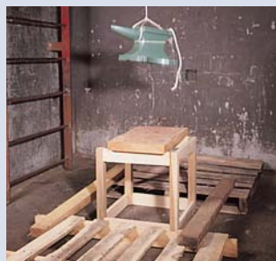
1) The anvil is about to hit the cube made using #20 biscuits.
