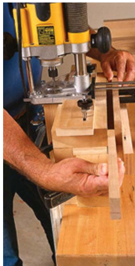
Here I'm cutting twin mortises. A spacer shares the channel with the edge-guide facing. With the spacer between the jig and the facing, the router can cut the first mortise. Moving the spacer behind the facing bumps the router out, so it can cut the next mortise.
