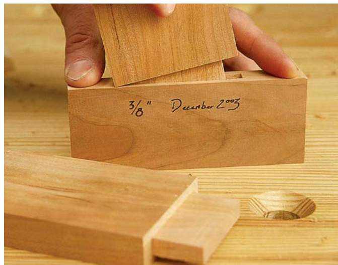
These sample mortises are useful for sizing your tenons. I usually make a new one every season or two, because they can get worn from use.
