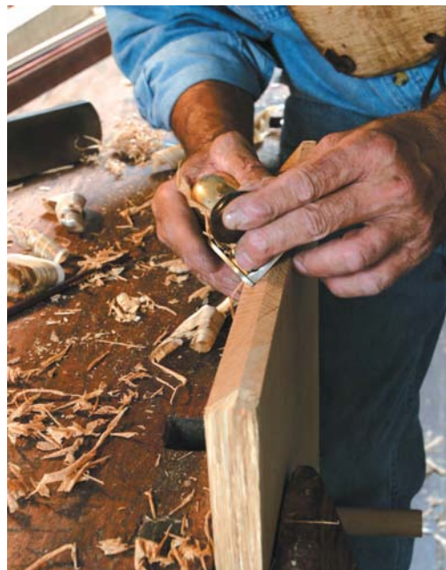
A sharp block plane excels at cleaning up saw-cut edges, whether they've been cut with a hand saw or an electric saw.
