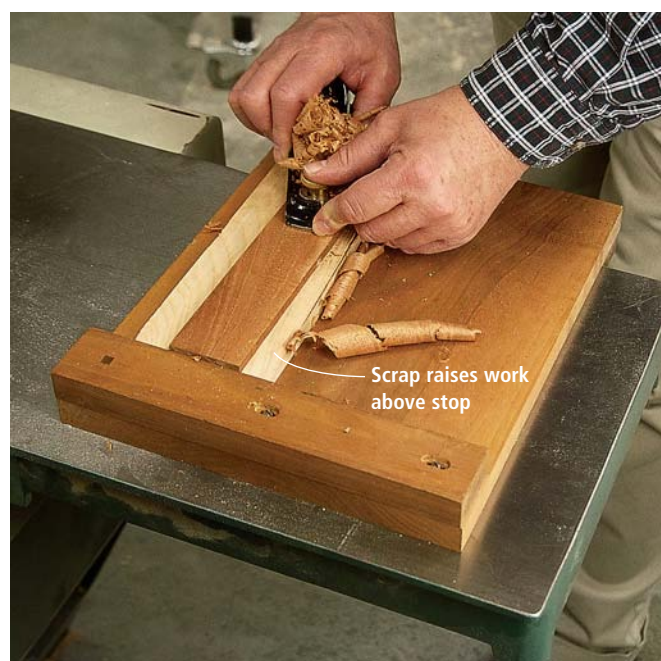
Bench hooks can be used almost anywhere (such as on the bed of this jointer) and can do some surprising tasks. Here it is being used as a small planing board. The light-colored scrap below the work raises the work above the bench hook's stop.
