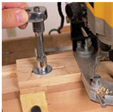
Position the bit at the mortise's end mark, slide the stop against the base of the router and secure the stop. Then repeat this at the other end.
