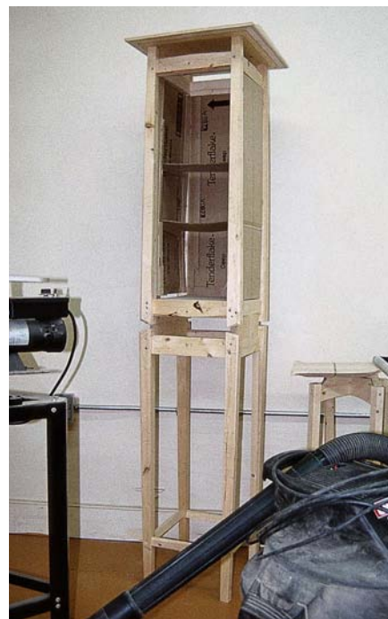
Once a mock-up is complete (such as this one), the student can make the full-size drawings necessary to build the project.
