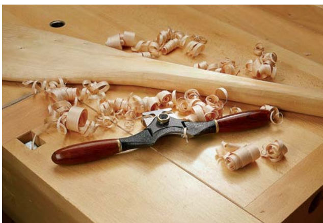
A spokeshave with a concave sole, such as this one from Veritas, excels at rounding the shaft of the paddle.
