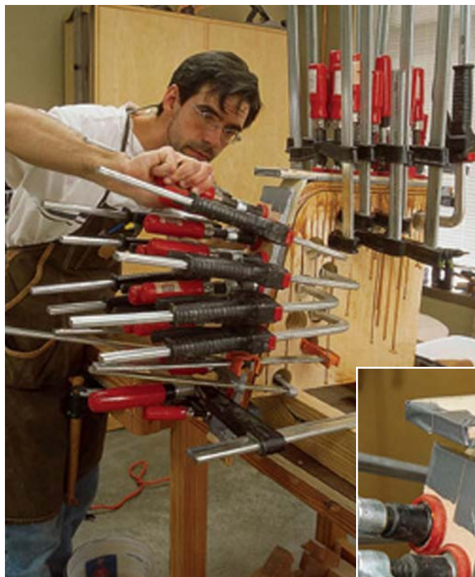
Turn off the radio, hold your calls and don't stop to chat during this part of the project. Speed and accuracy make a good lamination. This glue can set up fast.
