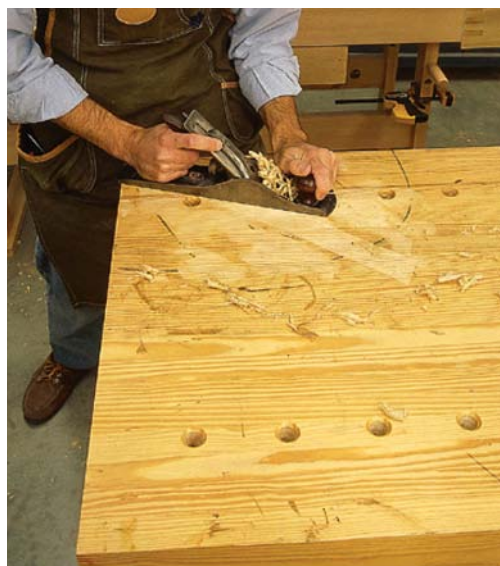
Most of the hard work when flattening your top is handled by the No. 5 jack plane, which can take down high spots quickly. My bench always seems to dish in the middle (similar to a waterstone), so I begin by taking down the sides.
