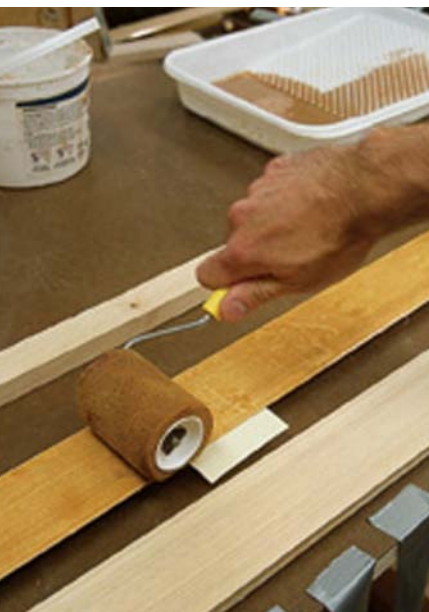
Don't use too much glue, or you will just make a sliding mess when the clamps go on. A thin film on both sides is enough to do the job. Dry spots on the plies are a no-no, however.
