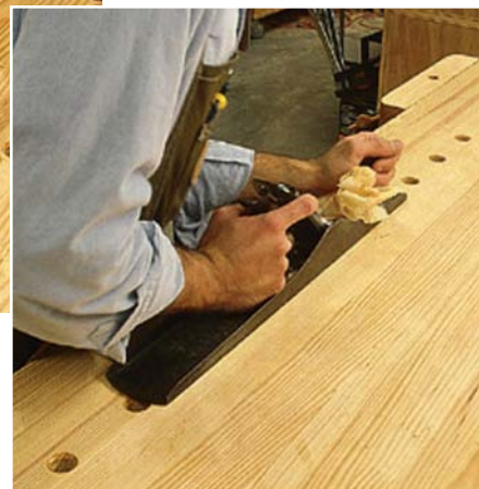
A No. 7 jointer plane's key asset is its length. Because of its length, the plane rides over the low spots and shears the high spots. Begin by working diagonally; don't worry about tear-out (above). When the top is flat from your diagonal passes, plane directly with the grain (right).
