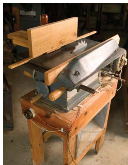
The Craftsman tilt-top table saw was revolutionary for the early '40s. All of today's table saws owe their lineage to this machine. We now tilt the arbor rather than the table, but it's nice to see the beginnings of such an important machine.
