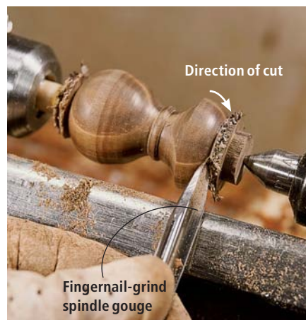
Refine the shape and make the finishing cuts with a long-fingernail-grind spindle gouge.
