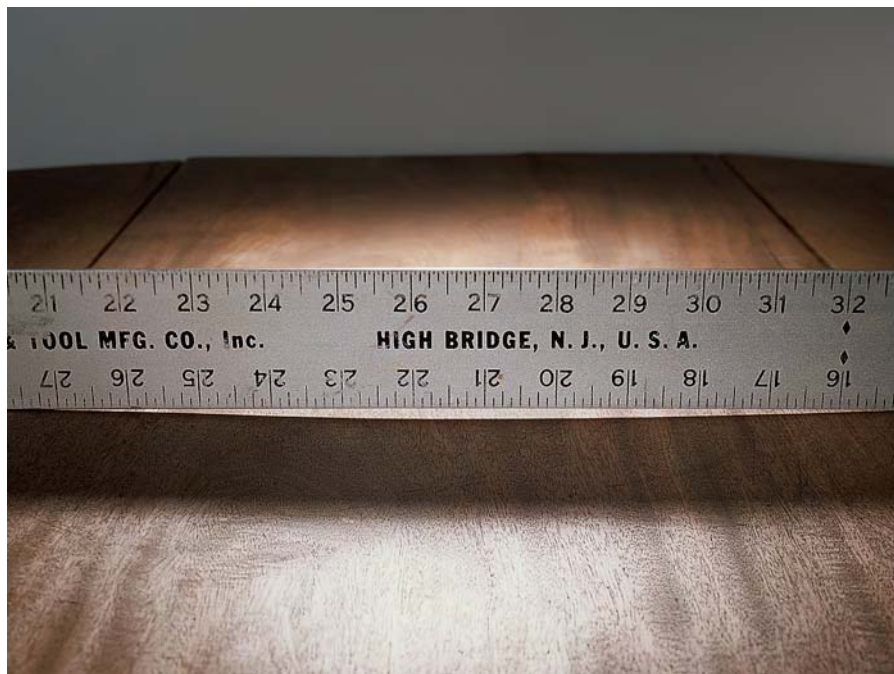
Old tabletops commonly cup on their tops even though the direction of the boards' rings and the fact that the bottom sides are often left unfinished would indicate that the opposite should have happened. The cause is compression shrinkage. The gap of light between the ruler and the wood indicates a warp.
