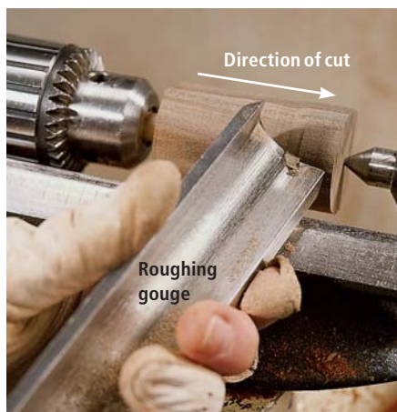
Round the workpiece with a roughing gouge.
