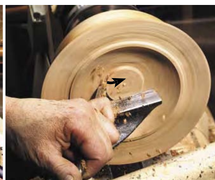
Note the position of the tool as I begin the cut. To keep the bevel rubbing while cutting the side of the bowl, the handle must be held far to the right and must swing around to the left as you cut to the bottom or center of the bowl.
