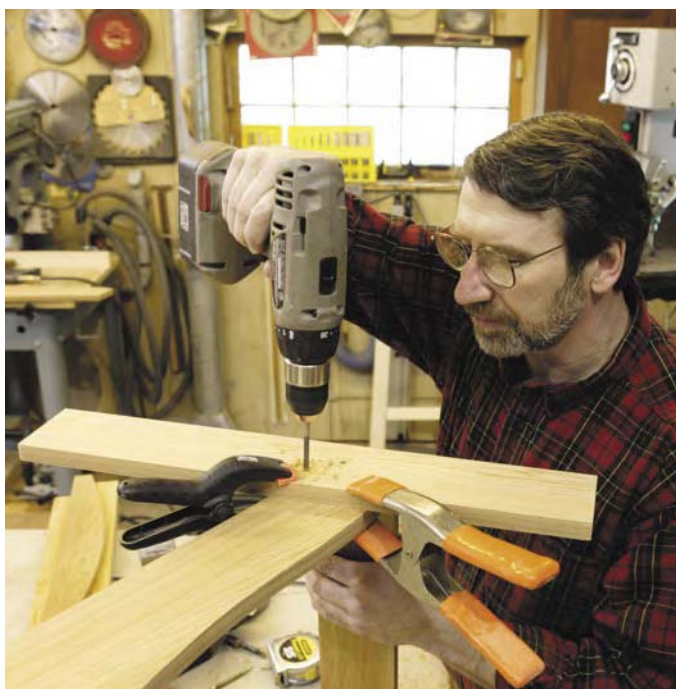
Arm installation over leg & bracket
