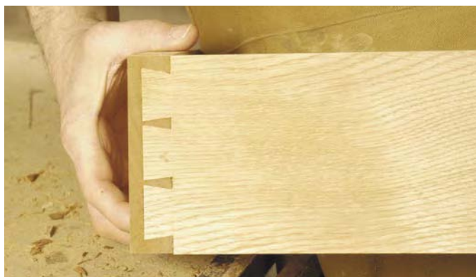
You're done. Parts should fit snugly, but if you find you have a gap between a tail and a pin, a sliver of wood and a touch of glue will work wonders.
