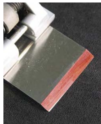
Here is what the corner of your iron will look like after about a dozen strokes. The shiny narrow triangle is where metal has been removed.
