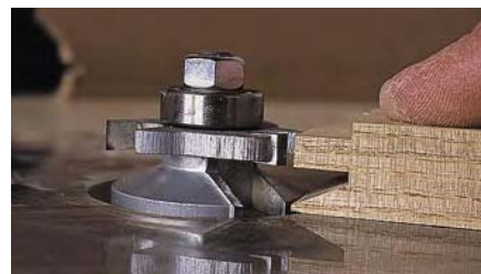
Use one of the coped pieces to set the height for the sticking cutter.
