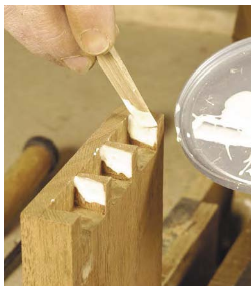
First test the joint by just starting the two pieces together. Pare away any material that would seem to interfere with the joint. Then apply a bit of glue to the sides of the pins and assemble the joint.
