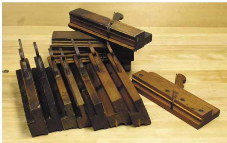
Technically, beads and sash planes (as shown here) are complex moulding planes, but they are rarely categorized as such.
