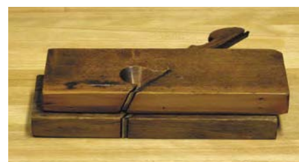
A skew rabbet plane (top) can work across the grain or with it. The square rabbet plane (bottom) is easier to freehand.
