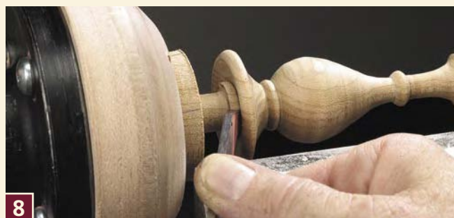
8 Make a wide, undercut flange and a \frac{1}{2} "-diameter tenon at one end.
