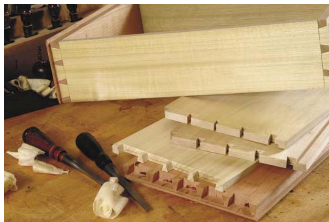
The lip on the drawer front, made from cherry, overlaps the frame of the cabinet when the drawers are completed.
