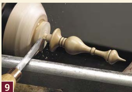
9 When sanded, finished and parted off at the narrow end, part it off at the end of the tenon.
