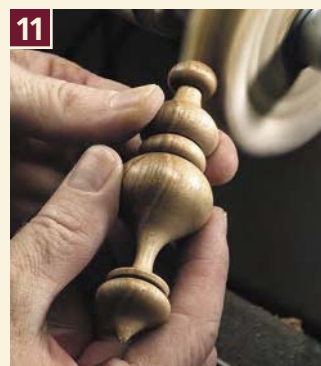
8 Make a wide, undercut flange and a \frac{1}{2} "-diameter tenon at one end.
