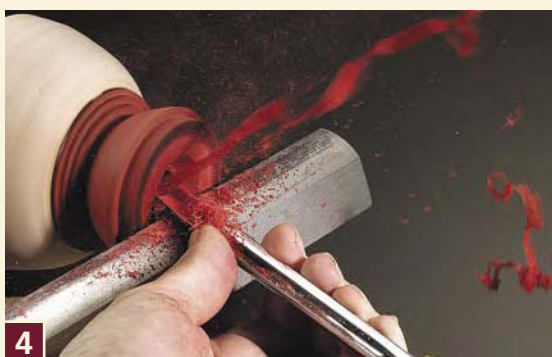
4 Hollow out the interior with a spindle gouge.
