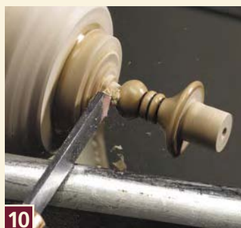
10 Make the short (top) spindle or finial.
