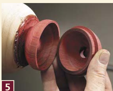
5 Here I have mounted the second half, cut a recess to fit the first half, and hollowed out the interior.
