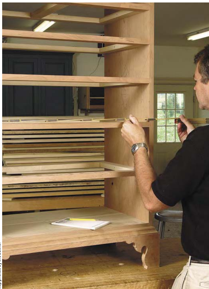
Carefully measure the openings for the drawers to achieve a precise fit of the drawer box. Add for the lip to determine the exact size of the drawer front.
