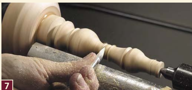
7 Mount and turn the long (lower) spindle. This is just like turning the icicle ornament; see those instructions for more detail.
