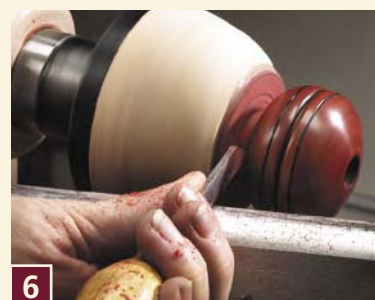
6 Glue the halves together and complete the exterior; sand, finish and part off.
