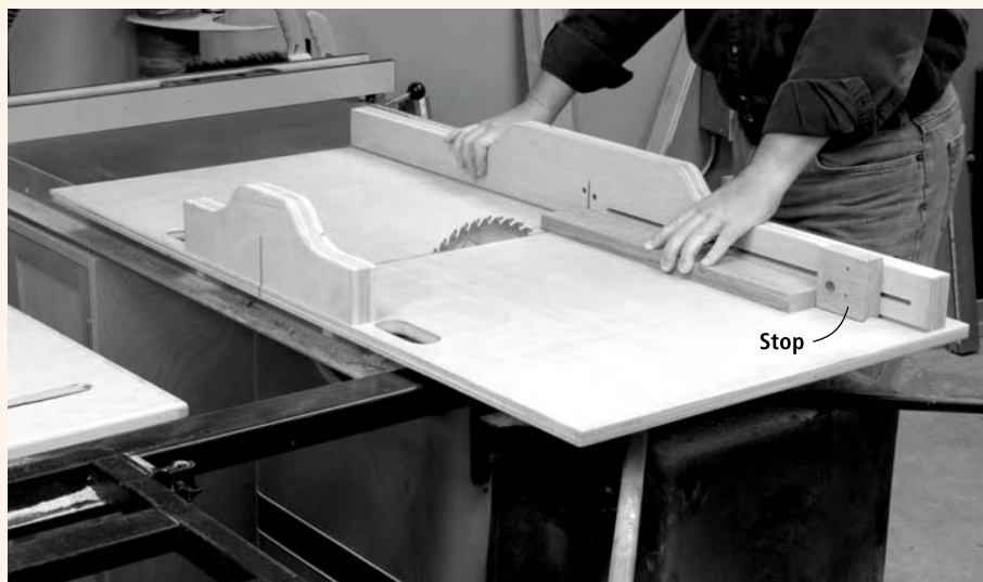
A two-sided miter sled allows equal support on either side of the blade and also functions as a partial blade guard. While stops can also be added into this design (as shown) it doesn't easily allow for adjustable miter cuts.
