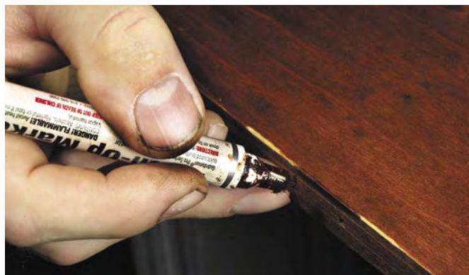
Touch-up markers are very effective on scuffed-up sharp edges. They are available in a variety of colors. To best match your piece, do a sample piece first.
