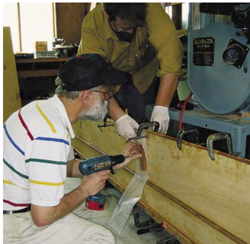
In a 12'-long boat, the plywood must be scarf joined for length. The long beveled overlap joint uses scrap blocks on each side squeezed together with deck screws. Merlin (left) and Rick Eisenlord use waxed paper to prevent the blocks from being epoxied to the hull, as you see here.
