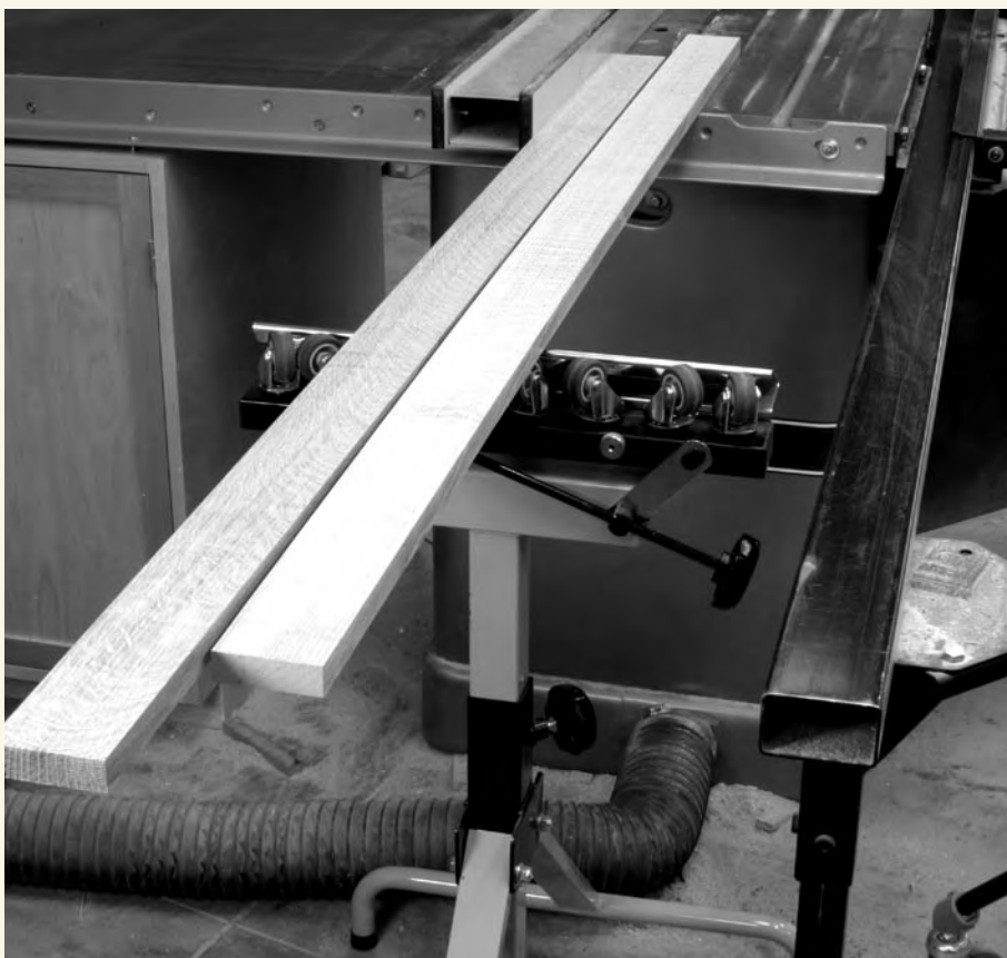
Roller stands serve as a simple helping hand when working with wide or long material. The Lee Valley stand shown here uses swiveling casters to support and move the material. It's adjustable for height in both gross or fine increments using separate mechanisms.
