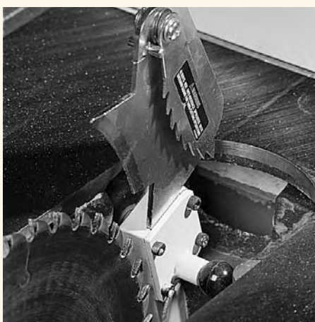
An aftermarket splitter/pawl assembly is shown in position (left) and being easily removed (right), without the use of tools. The splitter keeps a cut board from pinching the blade, while the pawls reduce kickback. The two parts work together to ensure your safety.
