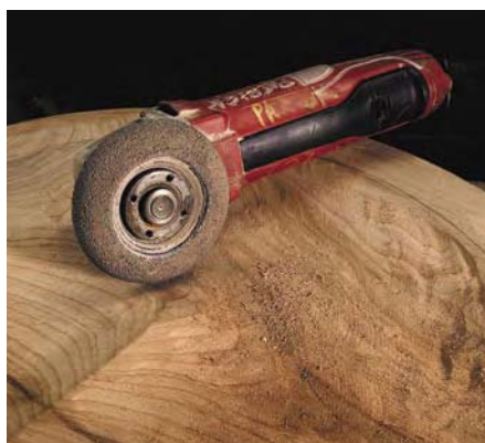
After the Arbortech, I clean up my work with these abrasive wheels, which come in different grits.
