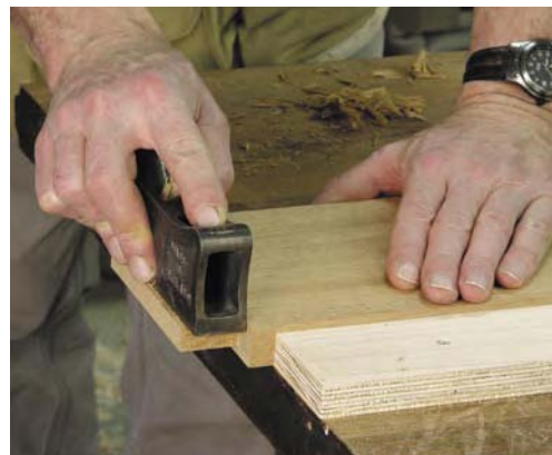
The tenons are adjusted to fit with my shoulder plane. A piece of scrap plywood attached to the bench acts as a bench stop to hold the work.
