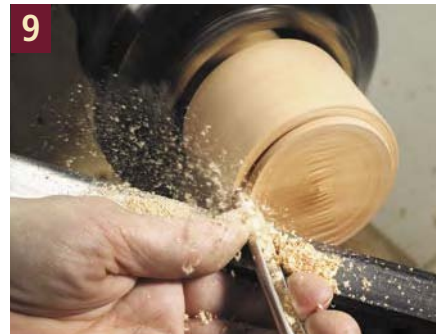
Cut the shoulder where the lid will fit.
