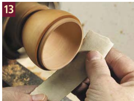
Sand very lightly to do the final fitting of the lid. It's very easy to take off too much, so use fine sandpaper and test the fit often.
