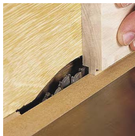
A rabbet cut into each edge of the board forms the tongue. It's smart to cut a sample and check its fit before cutting all your work.
