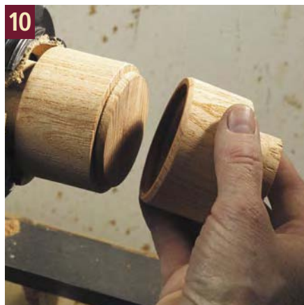
Test the fit. The lid should fit very snugly so it will stay on as you shape the outside of the box.
