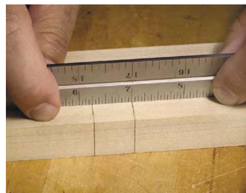
To deter parallax, position your rule on edge and view the numbers you're marking head on, as shown here.
