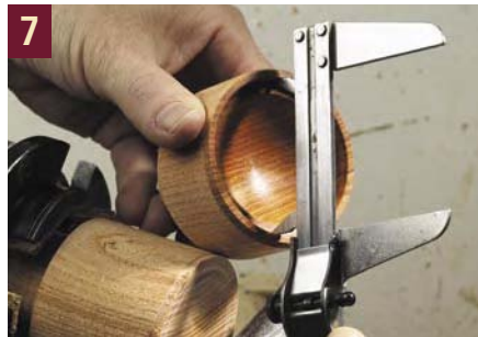
Measure the inside diameter of the lid with a metal caliper.
