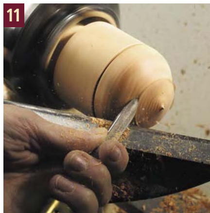
Turn the outside of the lid. Make small cuts and try to avoid catches, or you may pull the lid off.
