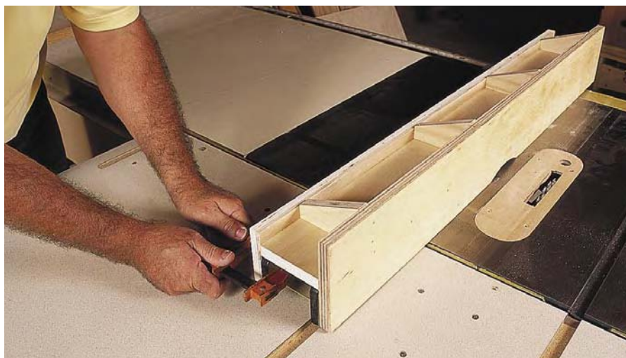
A sacrificial facing on the rip fence preserves the dado cutter and the fence, yet allows cut width adjustment using the fence position. More than just a facing, mine straddles the fence; one out-of-the-way clamp immobilizes it.
