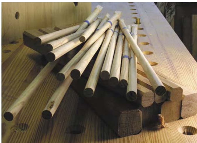
The sticks are kiln-dried ash; the leg blanks are kiln-dried oak. By sawing them out by following the grain lines of the wood I was able to get reasonably sturdy and workable stuff.
