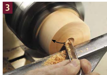
Begin hollowing the lid, using the fingernail-grind spindle gouge.
