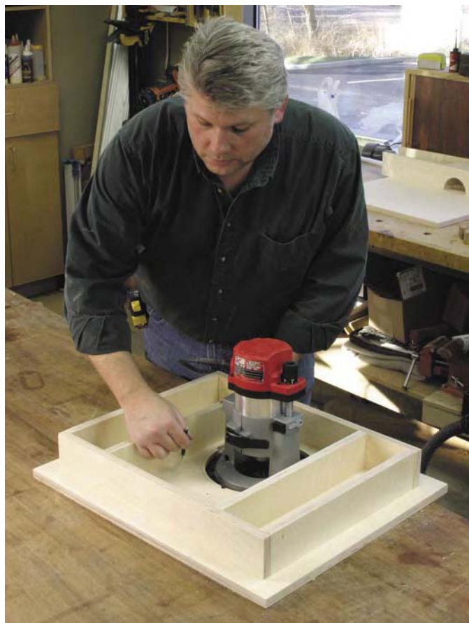
Allowing the proper clearance for your router is critical. You can see that I've removed the handles from the tool to allow as much space as possible. Mark out the space and then assemble the frame to fit.
