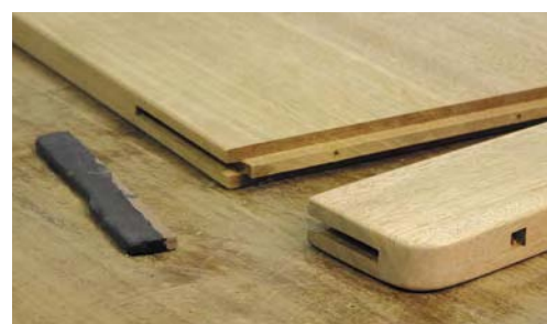
Breadboard-to-top connection
