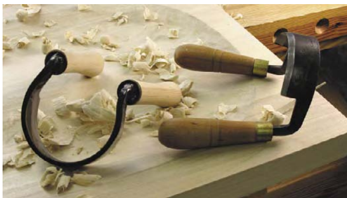
Traditionally, the inshave is used after the seat is roughed out with an adze. But my experiments found that the seat can be roughed out by an inshave alone. It takes a little more time, but is a good option until you find (or can afford) a proper adze.
