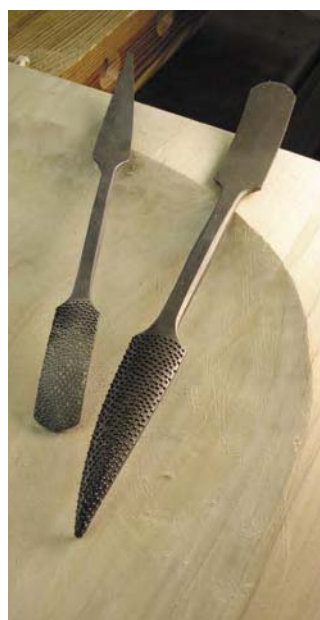
Curved rasps are great for many parts of the chair, from removing tear-out in a seat to shaping the outside of the seat, the bow and the comb. Their strength is they can detail curves and work (in general) without regard to grain direction.
