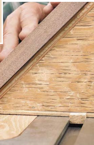
Each mitered end of the aprons receives a slot for the splines. The completed joint is strong, even though the splines are thin (inset).
