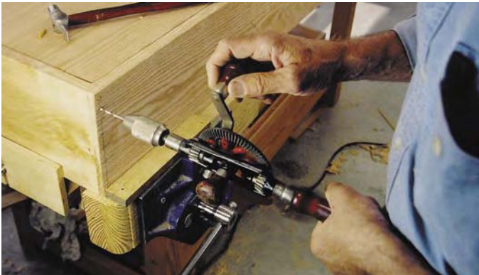
Here I’m using a hand drill (sometimes called an eggbeater drill) to bore the pilot holes for my locust pins.
