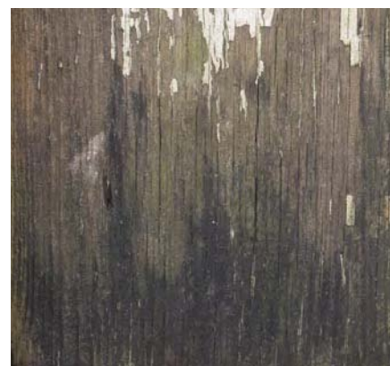
The mildew on the lower part of this board is a dark fungus that develops in moist conditions, especially in sheltered areas away from sunlight. You can prevent mildew by applying a wood preservative or a coating that contains a preservative. You can remove mildew by power washing or applying household bleach diluted with two to four parts water. Mildew causes little harm to the wood, but it looks bad.
