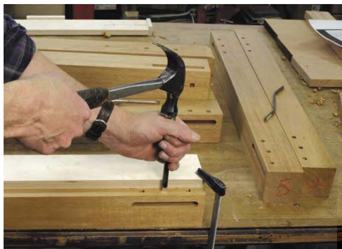
A modified chisel from a hollow chisel mortiser turns round holes square with just a few hammer taps. Plywood clamped to the leg keeps the chisel straight.
