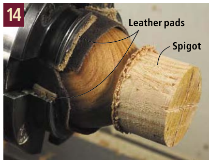
Re-mount the box in the chuck to turn off the spigot. Use fairly thick, stiff leather to cushion the finished box from the jaws.
