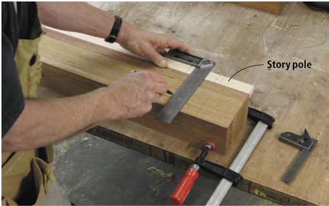
With the dimensions marked on a story pole, the locations for the mortises are marked on the legs as a group.
