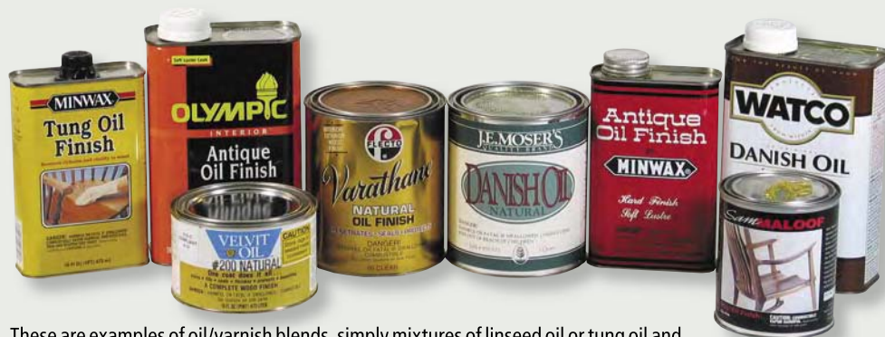
These are examples of oil/varnish blends, simply mixtures of linseed oil or tung oil and varnish, usually thinned with mineral spirits. You can tell that a finish is an oil/varnish blend if it contains mineral spirits and a puddle on top of the can or other non-porous surface takes days or weeks to cure to a very soft and usually wrinkled film.
