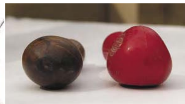
See the difference between the oval wood and the triangular-shaped piece of plastic. Bulbous, oval handles better distribute pressure.
