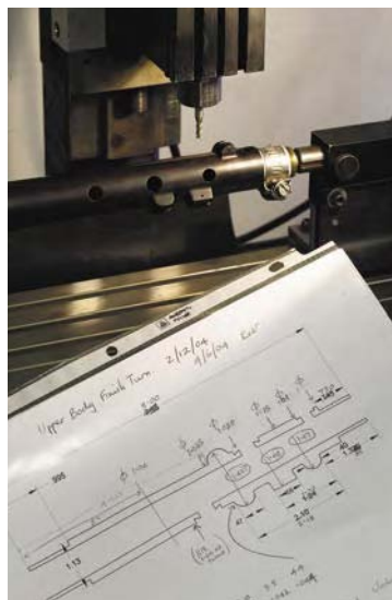
Copley uses a benchtop vertical milling machine made by Taig Tools to drill the keys and make the integral blocks for the buttons. Above you can see an illustration he uses for this process.
