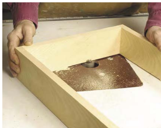
A rabbet for the back can be cut after the case is glued up with a bearing-guided rabbeting bit and a router table.
