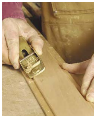
Chamfering the edges of the back boards with a block plane is a simple way of adding an attractive detail to the back.
