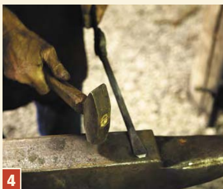
4 Steel can be made thinner. This technique, known as drawing out, allows the smith to take a piece of \frac{3}{8} "-thick steel, and thin it down to \frac{1}{8} " or less. Here I'm drawing out the pad of the holdfast.
