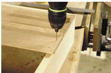
Drilling a pilot hole for 16-gauge brads will help prevent splits in these cherry back boards. The white pine case is soft enough to handle the nails without pilot holes. If screws are used, a full-depth pilot and countersink would be smart.
