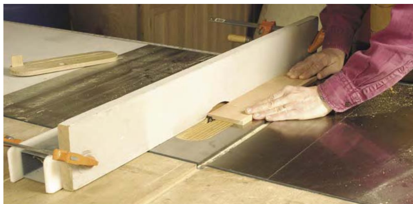
Shiplaps can be run off in a single pass.
