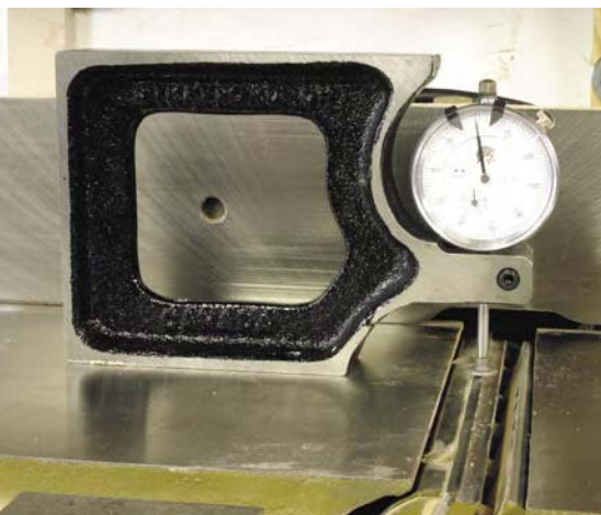
The Oneway Multi-Gauge sits solidly because of its mass, and the dial indicator can be turned to read it from any direction.
