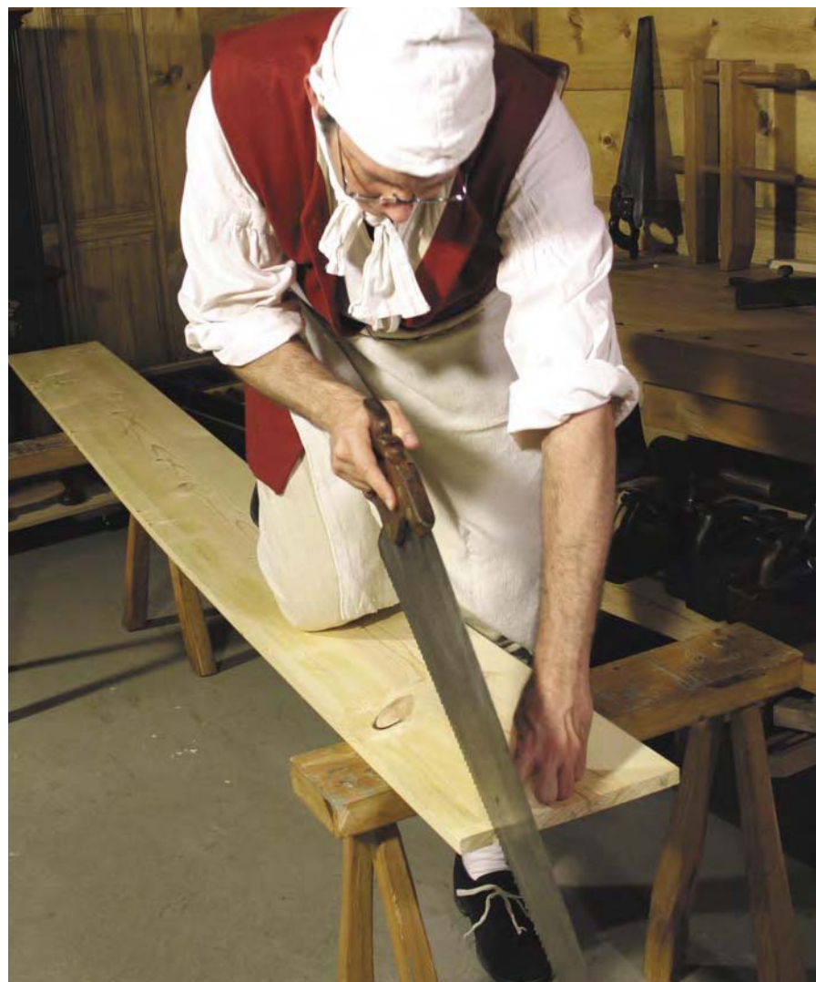
Ripping at the horse is surprisingly fast and effective. Here (dressed in the traditional garb I wear at Pennsbury Manor) I'm using the more heavily raked teeth at the toe of the saw to help start the cut.
