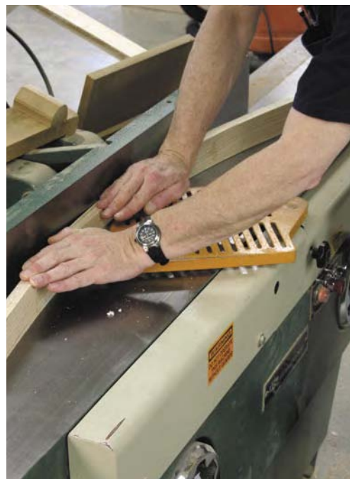
After scraping off the excess glue, one edge is evened up on the jointer. Make sure to keep the curve in contact with the fence on the outfeed side of the cutterhead.
