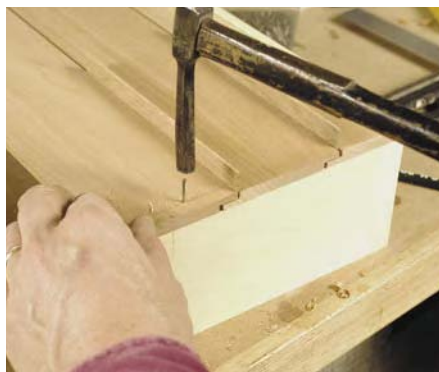
Two fasteners about 1" apart adequately hold each board in place.
