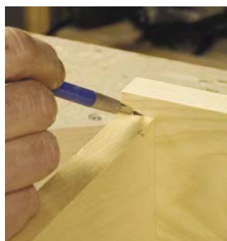
To mark the rabbet location, you can use a top or bottom piece to mark the inside of the cabinet side. The mark represents the height of the dado blade.
