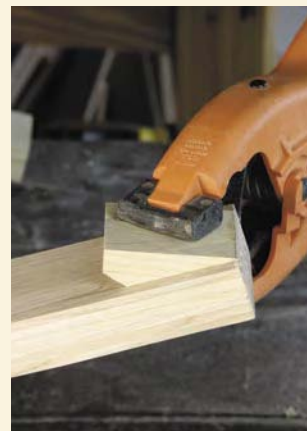
The other half of the hanger is glued to the back of the shelf support, letting the shelves hang nearly invisibly.
