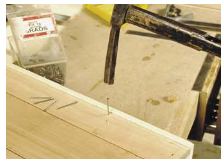
If boards used at each edge are narrow, they can be fastened directly to the rabbets cut in the sides of the case. This would help to strengthen larger cases but probably isn't necessary in small ones.
