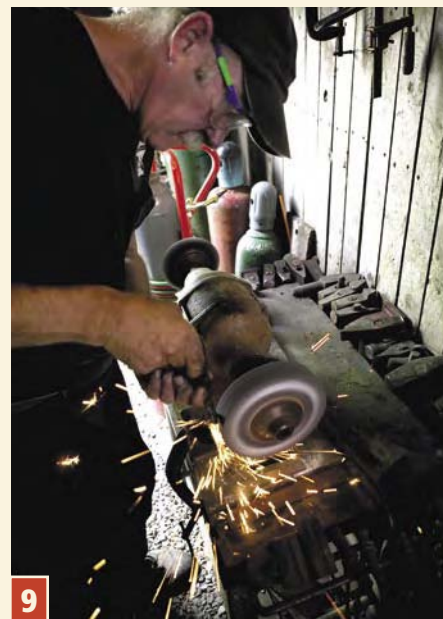
9 Grinding finishes the tool. If this were a cutting tool, I would then harden and temper the edge. But that step is unnecessary with a holdfast.
