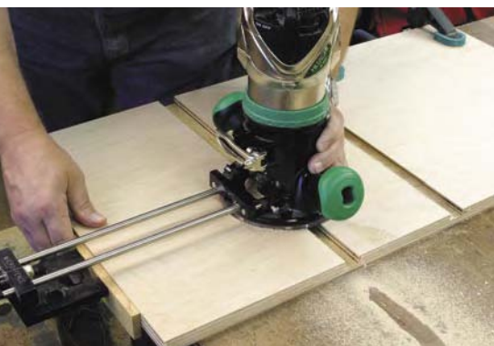
After making my centered 3/4" x 3/8"-deep dado, I cut both the side 1" x 1/2"-deep dados using two passes with the same bit.
