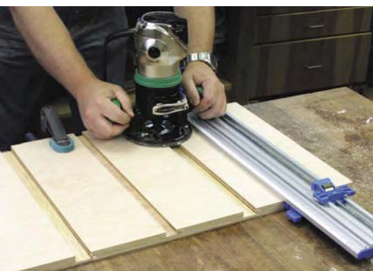
The second 1" dado must be parallel to the first, so if you use a router guide as shown here, measure carefully from the first dado to align the cut.
