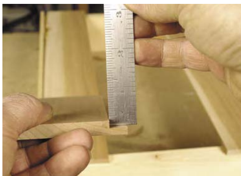
Before cutting the shiplap profile into the edges of the back pieces, try the table saw or router table setup on a piece of scrap first.
