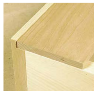
When the top and bottom of the case won't readily be seen, the top and bottom cabinet pieces can be made narrower than the sides allowing the back pieces to run the full height of the case.
