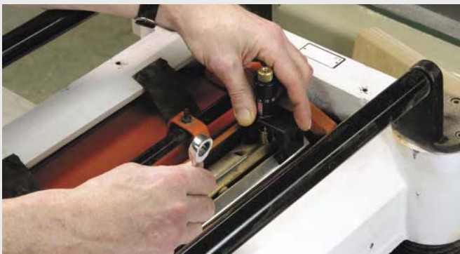
Tightening the knives can cause them to move away slightly from the cutterhead. Use a jig to hold them while tightening and always double-check your work afterwards.
