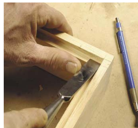
The router will leave rounded corners that can be squared up with a chisel. Alternately, shape the corners of the corresponding back pieces to fit.
