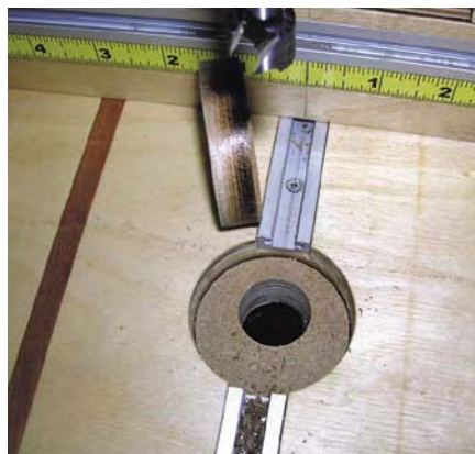
The two-plug system brings the insert flush to the table surface. Also notice the offset location (the through hole is where the bit will drill) to keep the discs from spinning.
