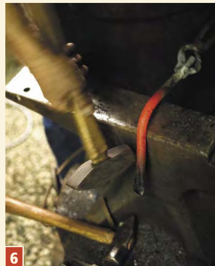
6 Steel can be bent, twisted and contorted. When it's hot, it's a plastic material, capable of being shaped into almost any form. Here I'm bending the holdfast into its optimal shape.
