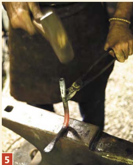
5 Sections of steel can also be made thicker. Here you can see I'm pounding the end of the shaft of the holdfast, which will thicken it where it bends at a right angle.
