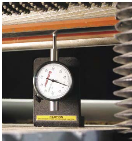
The Rotacator's compact size makes it ideal for measuring between the bed and the knives when setting up a planer.
