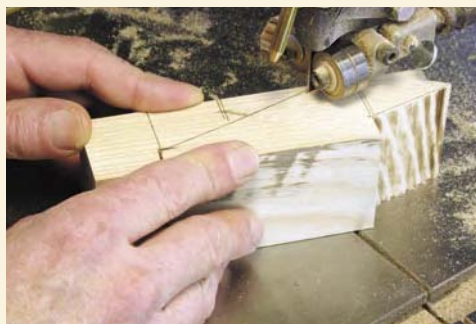
Cut the curve first, then make two short cuts to form the interlocking joint. The last cut frees the hanger from the block.
