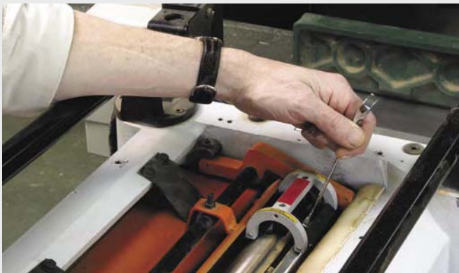
The easiest way to set the knife at the proper distance is to use a magnetic jig. Leave yourself room for the wrench when you position the jig.
