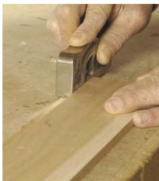
A rabbeting plane will remove any milling marks left from the dado and fine-tune the fit between adjacent boards. Each shiplap should end as one-half the thickness of the board.
