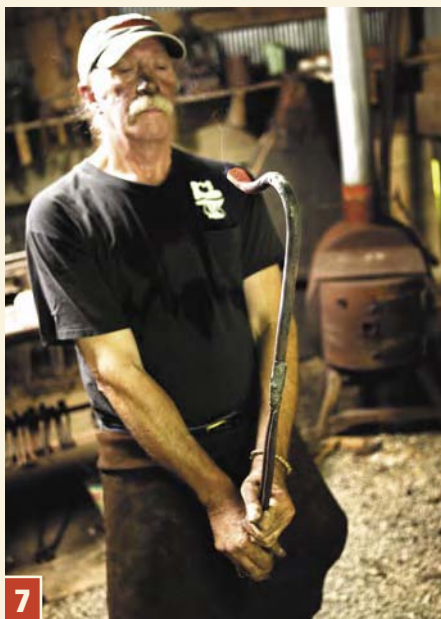
7 It's important to inspect for symmetry. Here I check to see that the pad of the holdfast is in line with the shaft.
